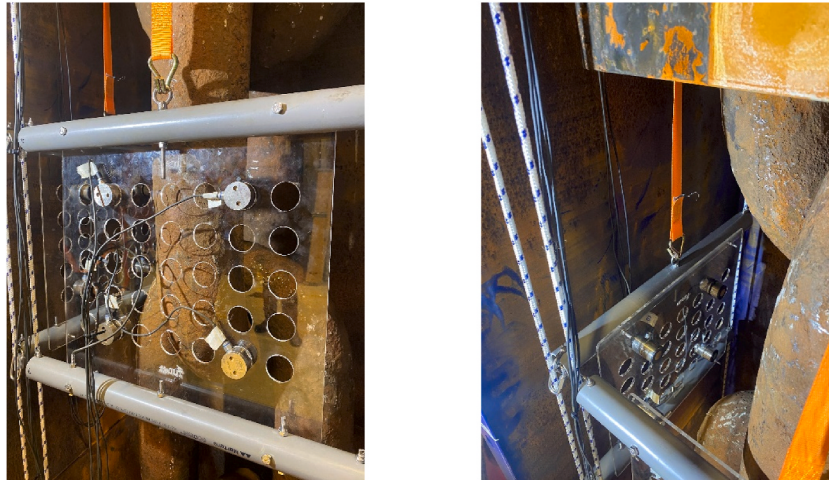
Fig. 4. Perpendicular movable arrays of AE transducers.
