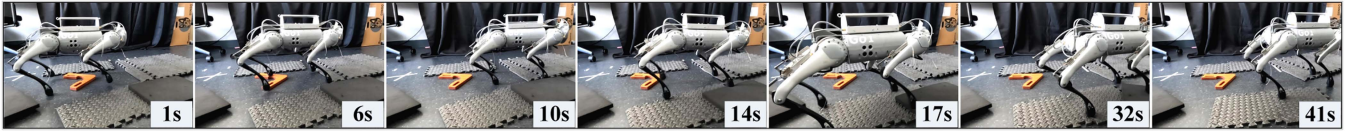
Fig. 13. E-Go walks across a collection of uneven terrains. None of these obstacles is known to the controller. The complete videos are available as a multimedia attachment.
