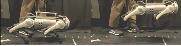
Fig. 1. Delft E-Go, the compliant quadruped with parallel elasticity, stores energy in springs (left) and releases it for an explosive jump (right).
