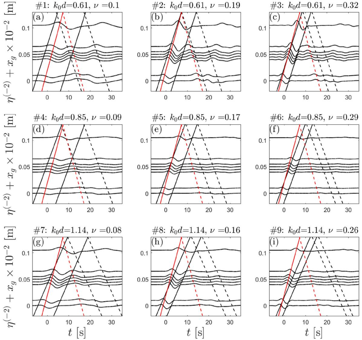
**Fig. 10.** For first-order accurate generation, spatio-temporal evolution of the sub-harmonic surface elevation at each wave gauge, vertically offset by the gauge location ( $x_g$ ). The continuous red lines indicate sub-harmonic error wave speed ( $c_e = \sqrt{gd}$ ), the black lines indicate the group width ( $2\sigma$ ), travelling at the group speed ( $c_{g,0}$ ); the dashed lines indicate their respective reflections.
