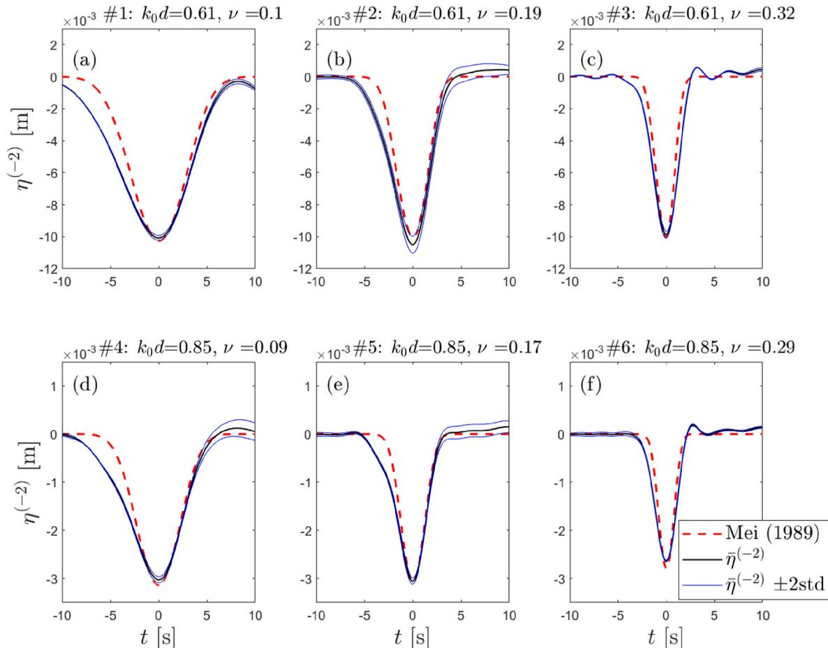
**Fig. A.13.** Sub-harmonic second-order generation repeatability in experiments 1–6. The mean of five repeats (black line), 2 standard deviations ( $\pm 2\text{std}$ ) around the mean (blue lines), the theoretical set-down according to Mei (1989) (red dashed line).
