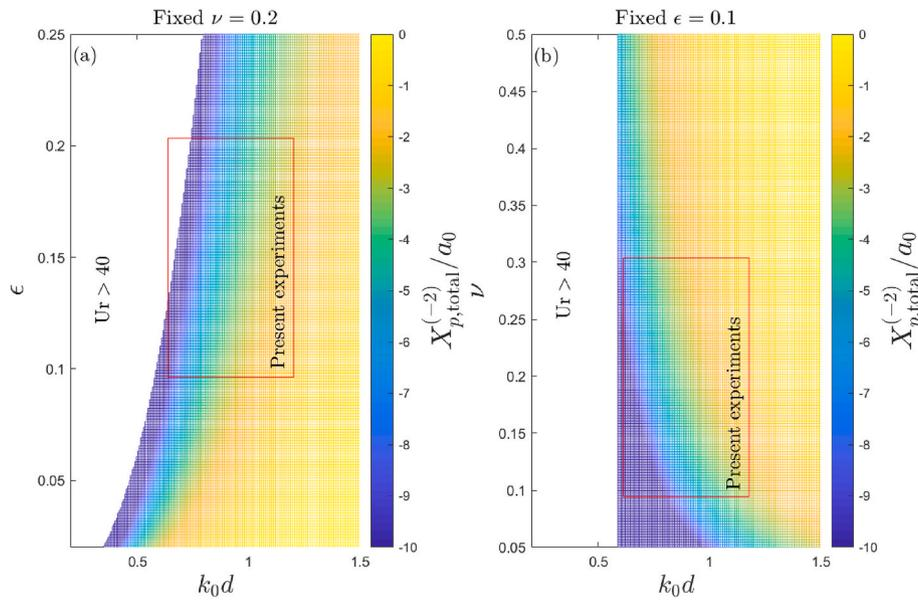
Fig. 5. Non-dimensional total backward paddle displacement: (a) as a function of relative water depth  $k_0d$  and steepness  $\epsilon$  for fixed bandwidth  $\nu$  and (b) as a function of relative water depth  $k_0d$  and bandwidth  $\nu$  for fixed steepness  $\epsilon$ . The present experimental range is indicated with red squares. The region in which the Ursell number is greater than 40 is blanked out and indicated as  $Ur > 40$ .
