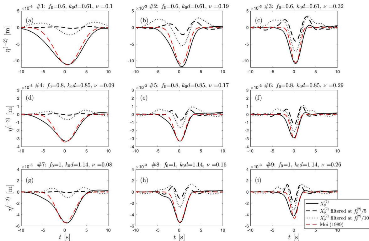
Fig. 8. The sub-harmonic measured surface elevation with second-order generation after filtering with the same high-pass limits as in Janssen et al. (2003).
