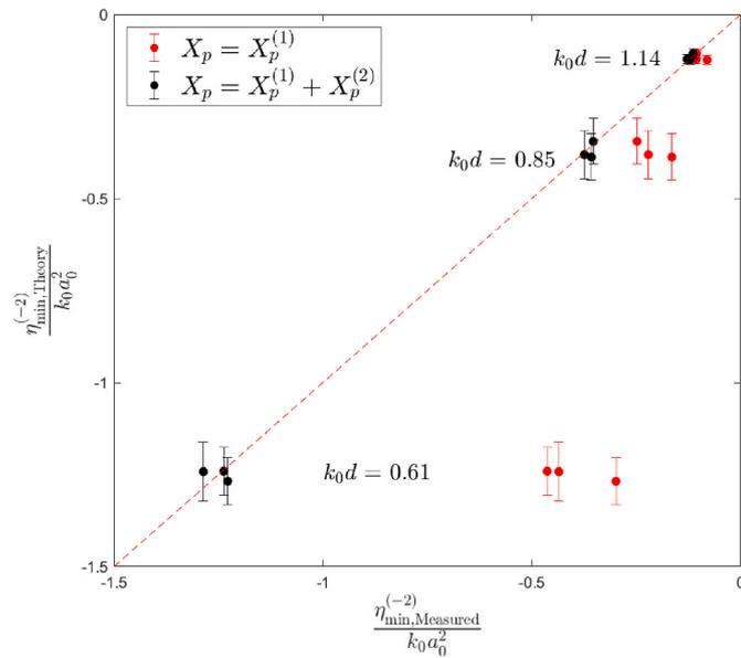
**Fig. 12.** Measured set-down amplitude  $\eta_{\min,Measured}^{(-2)}$  against the theoretical prediction  $\eta_{\min,Theory}^{(-2)}$  for all nine first-order and second-order generated cases. Error bars indicate  $\pm 2$  standard deviation around the mean, obtained from five repeats.
