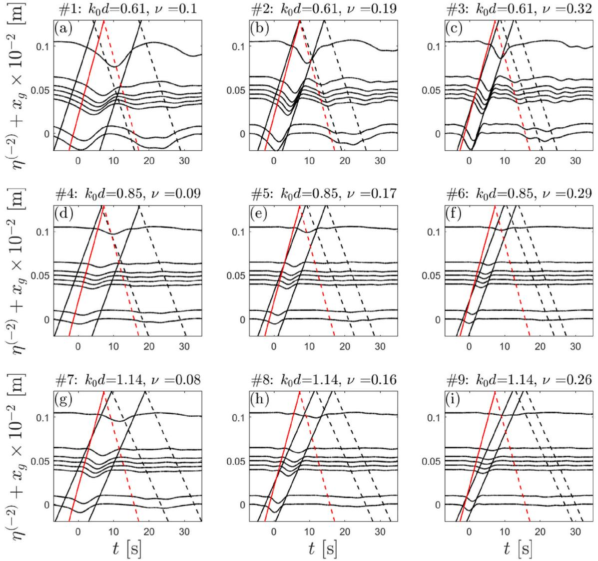
**Fig. 11.** For second-order accurate generation, spatio-temporal evolution of the sub-harmonic surface elevation at each wave gauge, vertically offset by the gauge location ( $x_g$ ). The continuous red lines indicate sub-harmonic error wave speed ( $c_e = \sqrt{gd}$ ), the black lines indicate the group width, travelling at the group speed ( $c_{g,0}$ ); the dashed lines indicate their respective reflections.
