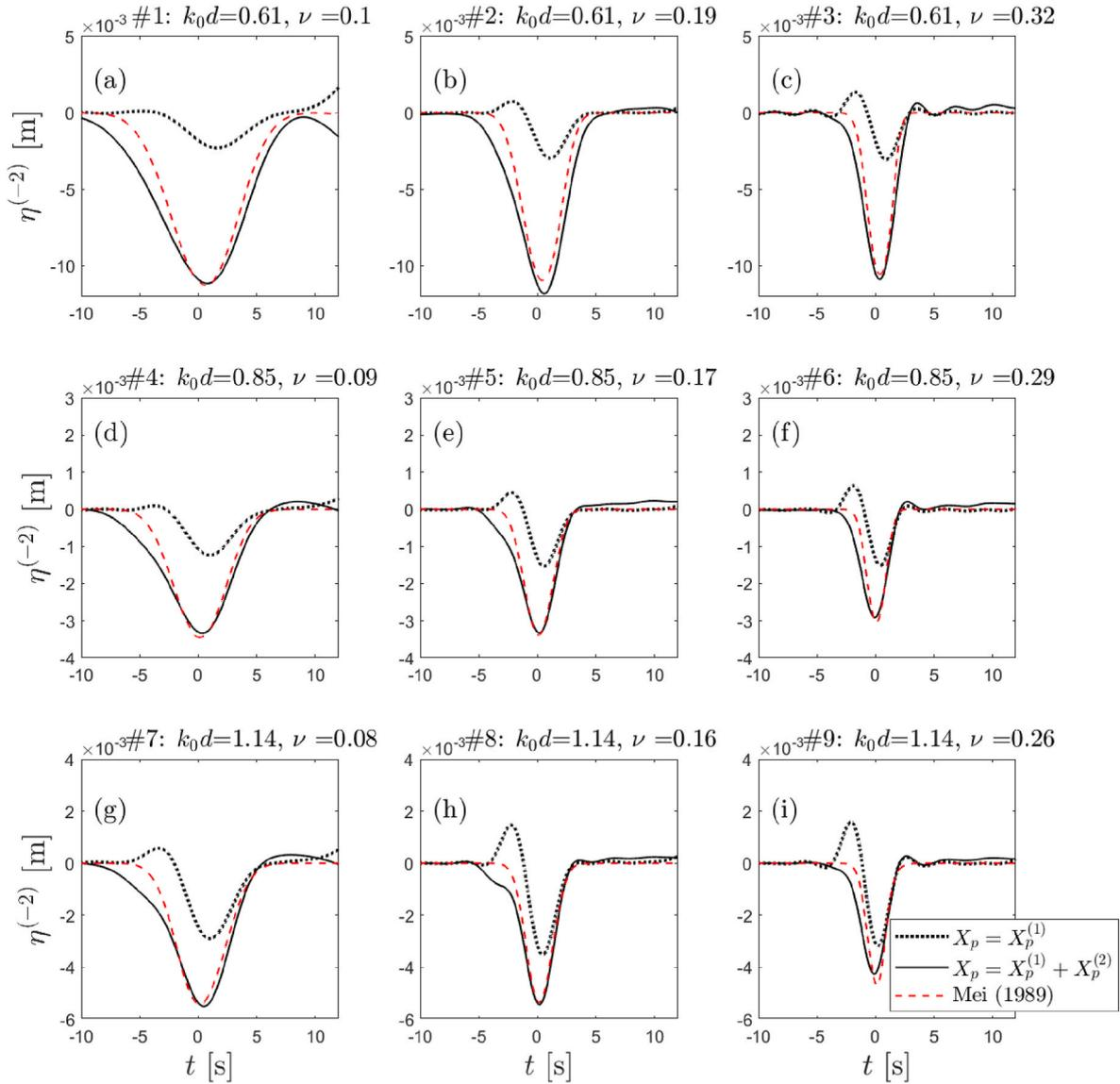
**Fig. 6.** Sub-harmonic surface elevation at wave gauge 2 for the nine experiments showing results for first-order generation (dotted black lines), second-order generation (solid black lines), and the theoretically predicted set-down of Mei (1989) (dashed red lines) computed using eq. (9).
