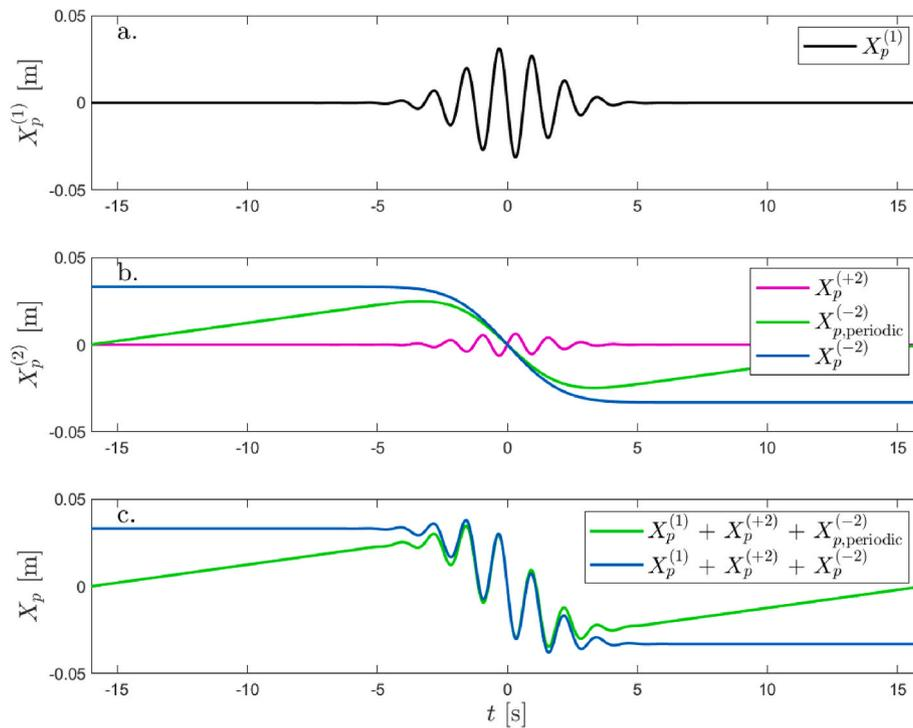
**Fig. 1.** Example second-order accurate wavemaker displacement time series for a Gaussian group: (a) first-order, (b) second-order, decomposed into super-harmonic  $X_p^{(+2)}$ , periodic sub-harmonic  $X_{p,periodic}^{(-2)}$  and non-periodic sub-harmonic  $X_p^{(-2)}$ , and (c) the complete second-order accurate wavemaker displacements.
