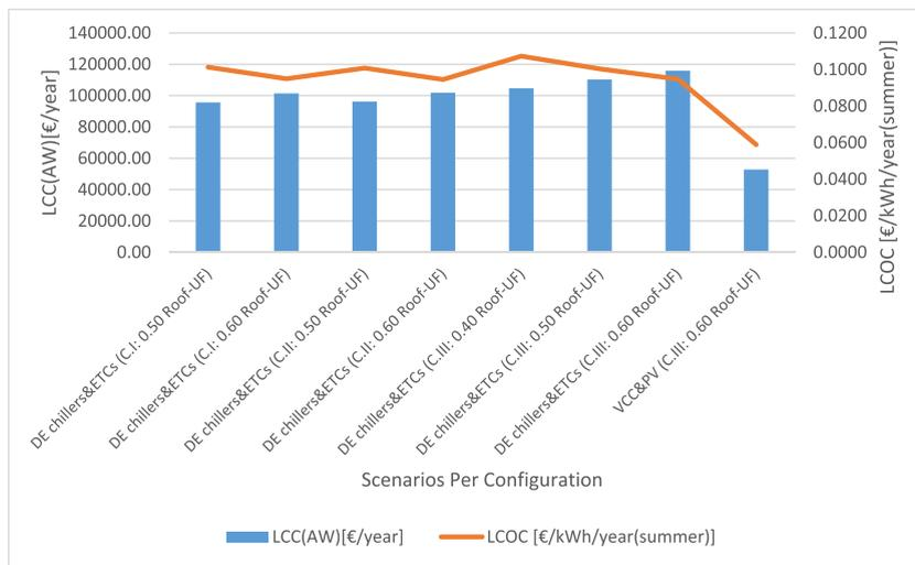
Fig. 6. Cost-effectiveness based on LCC<sub>AW</sub> and LCOC for scenarios involving Double-Effect (DE) absorption chillers with Evacuated Tube Collectors (ETCs) (thermally driven) and water-cooled VCC and PV panels (electrically-driven), considering those with Solar Fraction (SF) values of 1 or higher.
