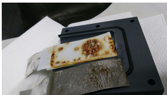
Figure I.1: Spot shaped corrosion on stainless steel.
