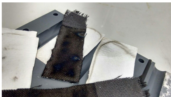
Figure I.3: Spot shaped 'burns' on carbon cloth.
