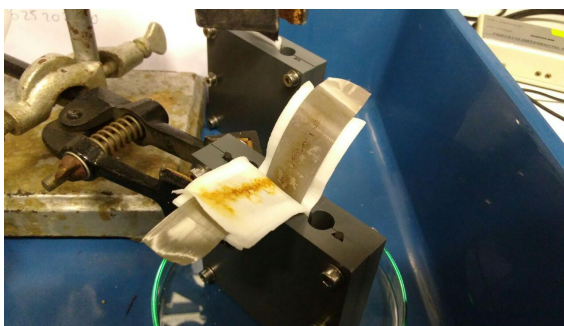
Figure I.2: Striped corrosion on stainless steel.
