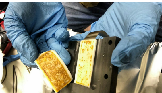
Figure I.6: Heavy corrosion over full steel surface.
