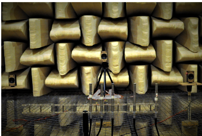
Fig. 10. Picture of the experimental setup considering five AVSs and three speakers, located at a radius of r = 3.6 m.
