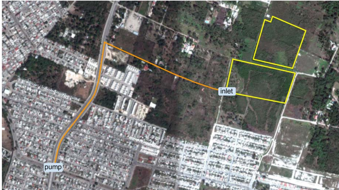
Figure 4.13: Pump and pipeline to infiltration basins in Presidentes de México
