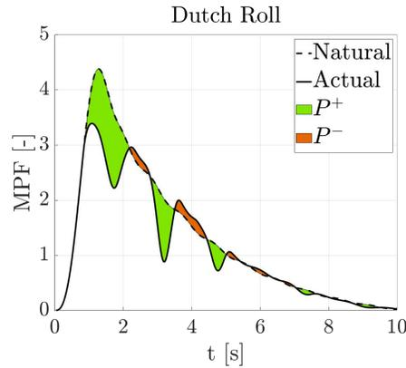
**Fig. 14 Visualization of Dutch Roll Suppression Performance**
