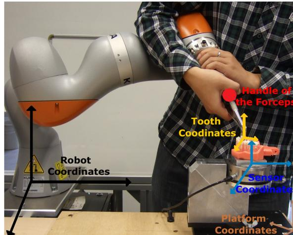
**Figure 4-1:** Four coordinates used in this project: robot coordinates (black), sensor coordinates (blue), tooth coordinates (yellow), platform coordinates (brown)
