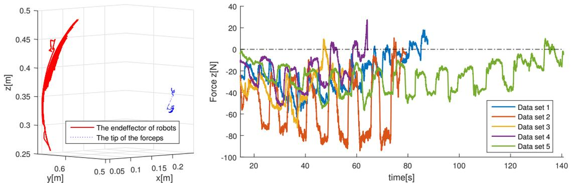
**Figure 3-3:** The figure one the left is the 3D trajectory of a human demonstration for tooth extraction. The figure on the right include the force in the vertical direction of multiple demonstrations
