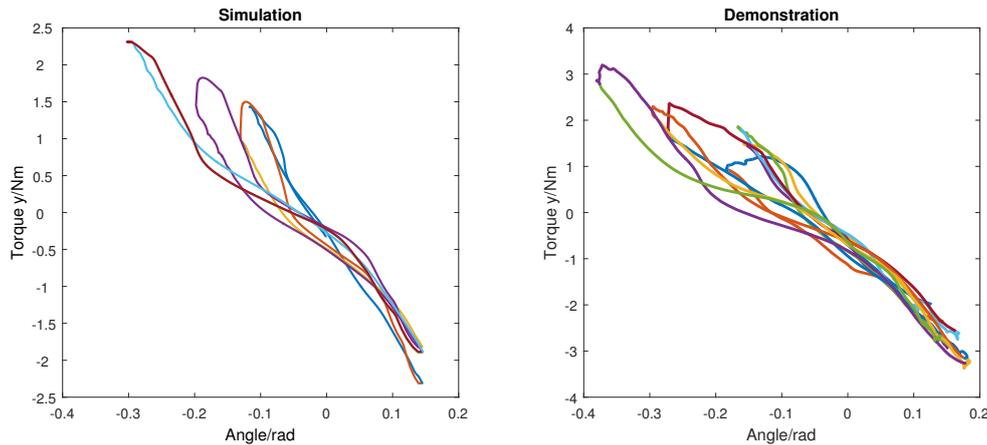
**Figure 8-4:** The comparison of the torque-angle relationship between simulation (left) and the demonstration (right). Different colors are used to distinguish different iterations of the movement. The overall trends are similar however, the details are different.
