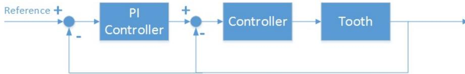
**Figure 7-3:** The flow chart of the controller level (robot controller).
