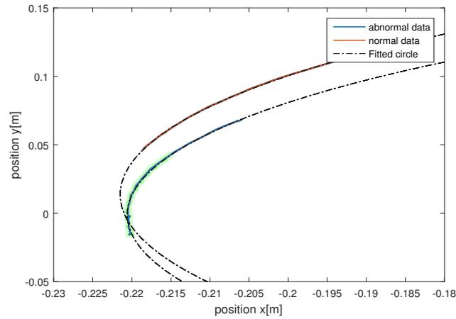
**Figure B-1:** The movement of the forceps in the demonstration with trend in  $F_y$  (red) and without the trend (blue). The shape highlights the area where the movement is no longer on the circle.
