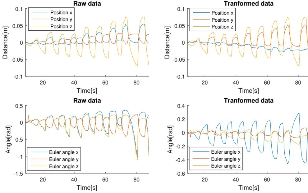
**Figure 4-2:** The position and orientation of the handle of the forceps. The upper part of the figure is the position data. The lower part is the orientation data. In addition, the raw data corresponds to the data on the left. The data after the coordinate transformation is on the right.
