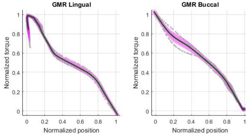
**Figure 5-5:** The learning result of the model of the reaction torque. The left part is the model on the lingual side and the other part is the model on the buccal side. The shade indicates the variance across different demonstrations.
