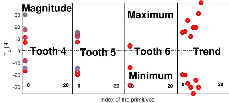
**Figure 6-6:** The maximum and minimum torque for every iteration grouped by the type of the tooth. Closely positioned points are the extremum for one type of the tooth. The color indicates different demonstrations. The horizontal axis in the local region is the index of iterations. The last group of point at the end of the figure is the maximum and minimum value of the trend for all demonstrations.
