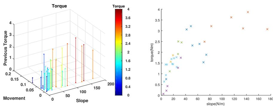
**Figure 5-6:** The effect of distance into the plastic region, the previous maximum torque and the slope of the correlation on the maximum value of the torque. The left part is the four-dimensional plot including all the factors. The torque is indicated by color. The right part is the plot of torque and slope after we identify a correlation between them in the left part.
