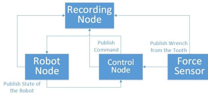
**Figure 7-6:** The Communication of different ROS nodes
