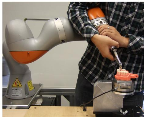
**Figure 2-2:** In the measurement setup. The robot is connected to the forceps and moves compliantly. The jaw is attached to the force sensor. The movement is recorded by the robot, and the interaction force is measured by the force sensor.
