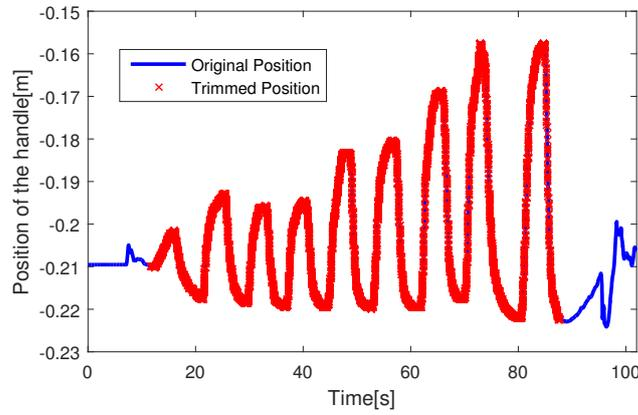
**Figure 4-3:** The blue line corresponds to the data with unrelated movements. The red cross represents the result of trimming based on the correlation in the demonstration.
