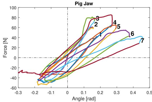
**Figure 5-1:** The correlation between the angle of the movement and the force  $F_y$ . The number is the order the contour is in the demonstration. The slope of the contour decreases over time. shapes are different in the positive and negative parts of the correlation.
