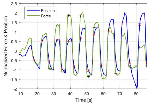
**Figure 4-6:** The result of the algorithm detecting all the change points. The change point in the position (red cross) corresponds to the start of the plateau of the force (black plus).
