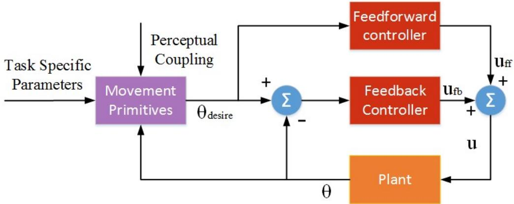
**Figure 2-3:** Control scheme with dynamic movement primitives [1]. The variable  $\theta_{desired}$  is the reference trajectory given by DMPs. The variable  $\theta$  is the sensed output of the plant. The variable  $u_{ff} + u_{fb} = u$  are the control input from feedback and feedforward controller.
