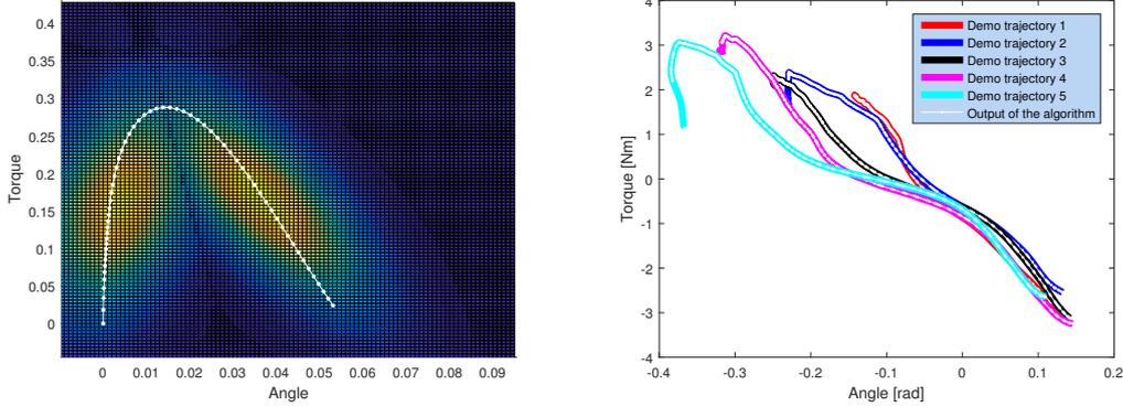
**Figure 6-11:** The model (left) and the result (right) of the algorithm that stop the movement after the ultimate strength. The shade color in the left part represents the probability distribution of the GMMs. The white dots are the trajectory that is used to train the model. The right part is the detection result of the demonstrations. Different colors represent different iterations. The white line indicates the region that the algorithm allows the robot to move.
