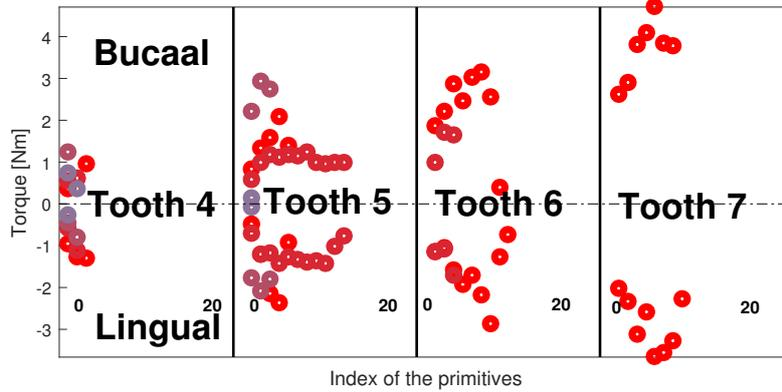
**Figure 6-4:** The maximum and minimum torque for every iteration grouped by the type of the tooth. Closely positioned points are the extremum for one type of the teeth. The color indicates different demonstrations. The horizontal axis in the local region is the index of iterations.
