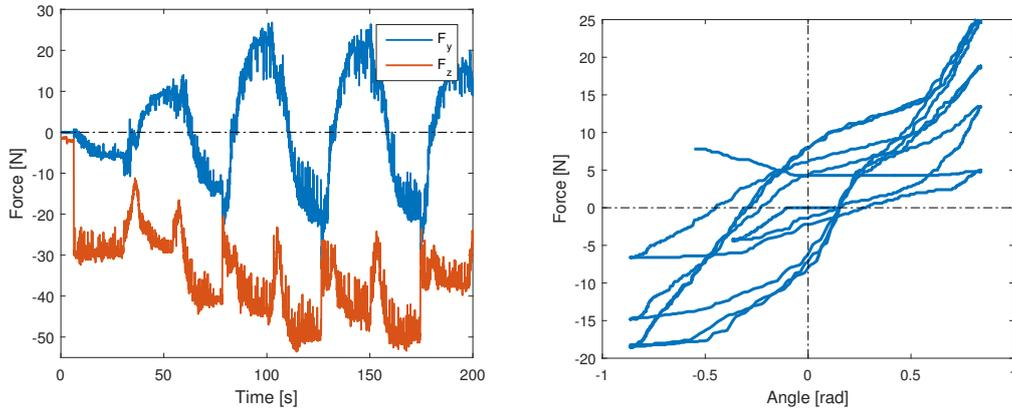
**Figure 8-6:** The left part of the figure is the comparison of the force  $F_y$  (blue) and  $F_z$  (red). There is no trend observed in  $F_y$ . The right part of the figure is the relationship between  $F_y$  and the angle. We can see a drop of the slope indicating the tooth is getting loose.
