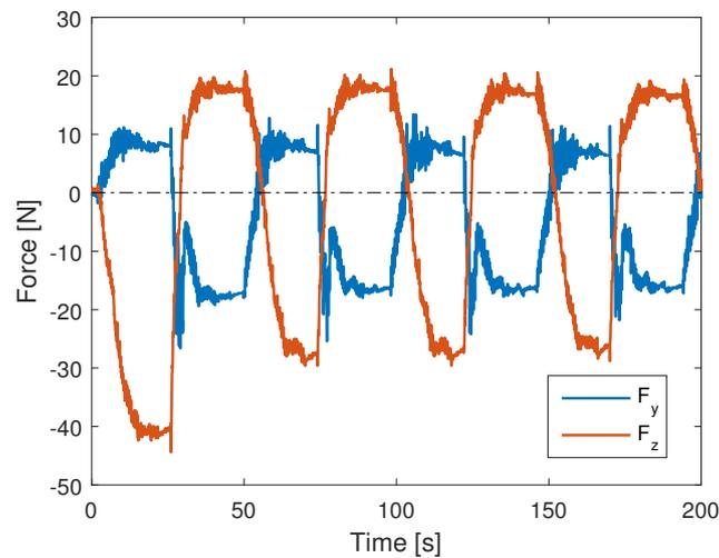
**Figure 8-7:** The force  $F_z$  (red) and  $F_y$  (blue) experiment without  $F_z$ . There is still a force  $F_z$  with relatively large value even though the robot apply no force in the vertical direction.
