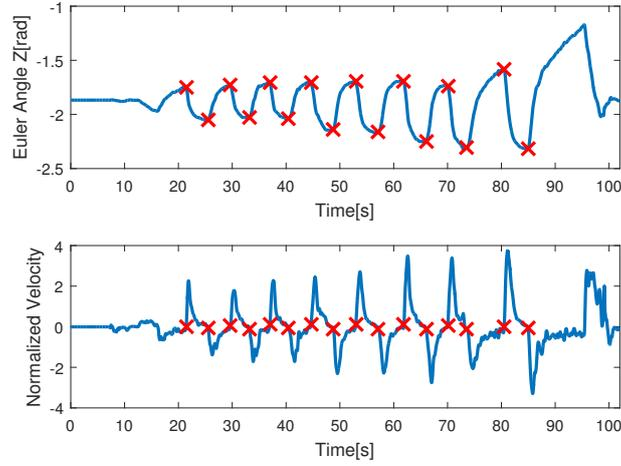
**Figure 4-4:** The result of the segmentation based on the change of the direction in the movement. The upper part is the movement, and the lower part is the velocity (cost function). The red cross indicates the point where the absolute velocity becomes larger than zero.
