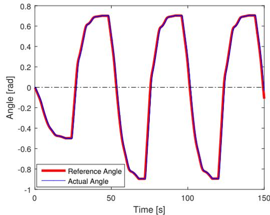
**Figure 8-5:** The reference tracking of the initial experiment on the robot. The red trajectory is the reference. The blue trajectory is the actual position of the robot
