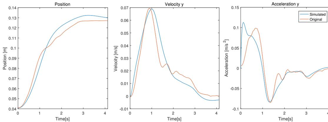
**Figure 6-7:** The position (left), speed (middle) and acceleration (right) of DMPs reproduction with ten radial basis functions for one demonstration. The reproduction (blue) has similar but smoother speed comparing to the demonstration (red).
