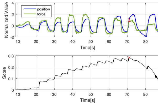
**Figure 4-5:** The result of one-change-point detection of the position data. The upper part is the comparison of movement and the force along its direction. The force (green) has a different shape on the top of every iteration. The cost function in the lower part of the figure shows that there are a lot of local maximums corresponding to each iteration of the movement. The red marks indicate that the positions of the change point in the position, the force and the cost function.
