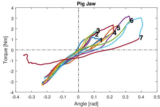
**Figure 5-3:** The correlation between torque and angles. The change of slope is observable on the lingual side because of the large force  $F_y$ . In addition, there is a decrease in torque with increasing position at the end of the movement on the lingual side. This corresponds to the ultimate strength in Figure 5-2.
