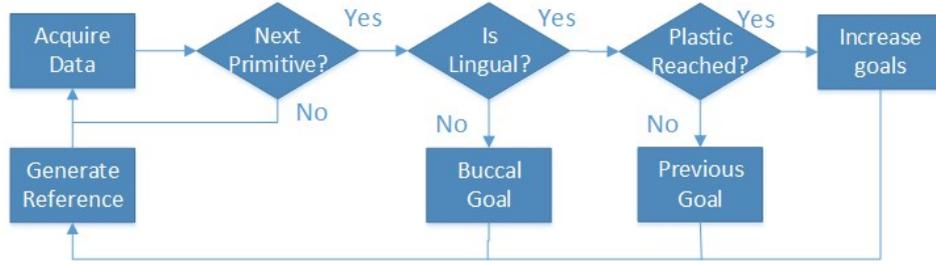
**Figure 7-2:** The flow chart of the decision level (High-level controller).
