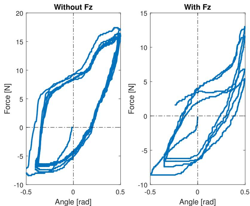
**Figure 8-8:** The comparison between the experiment with (left) and without  $F_z$  (right). The experiment with  $F_z$  results in a slope decrease in the model which means that the tooth becomes loose.
