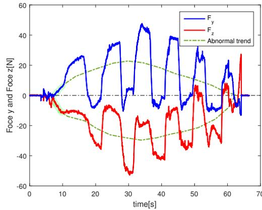
**Figure 3-4:** The comparison between the force in the vertical direction (red) and the force along the direction of the movement (blue). The green shade represents the start of the trend when the movement has not started. The green dash line is the estimated trend of both forces.
