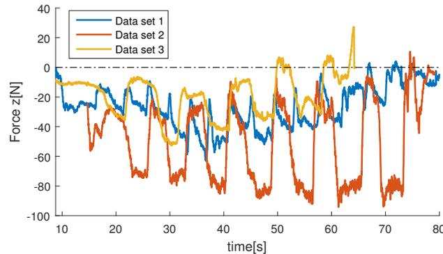
**Figure 6-5:** The vertical force with respect to time in multiple demonstrations indicated by different color
