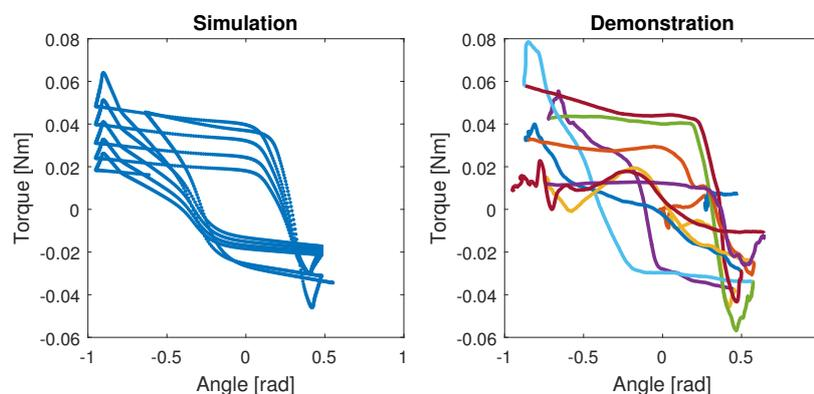
**Figure 8-2:** The response of the simulated plastic jaw (left). It has a similar shape and the change of the slope to what in the demonstrations of the plastic jaw (right). Different colors indicate different iterations of the movement.
