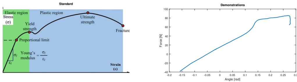
**Figure 5-2:** The figure on the left is an example strain-stress figure in the literature [2]. Comparing to the demonstration on the right, the plastic (green) and elastic region (blue) on the left have corresponding parts on the right. The ultimate strength is also clear which is at the end of the movement.
