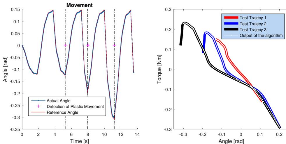
**Figure 8-3:** The left part is the tracking result of the simulation on the pig jaw. The actual position (blue) track the reference (red) successfully with the stopping point identified (magenta plus). The right part of the figure is the result of applying the algorithm that stops the movement after the ultimate strength. Different colors represent different iterations of the movement. The white line indicates the region that the algorithm allows the robot to move.
