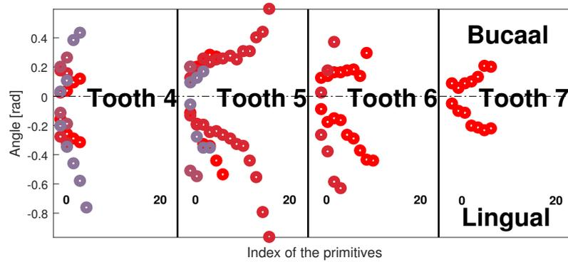
**Figure 6-2:** The maximum and minimum movement for every iteration grouped by the type of the tooth. Closely positioned points are the extremum for one type of the tooth. The color indicates different demonstrations. The horizontal axis in the local region is the index of iterations.
