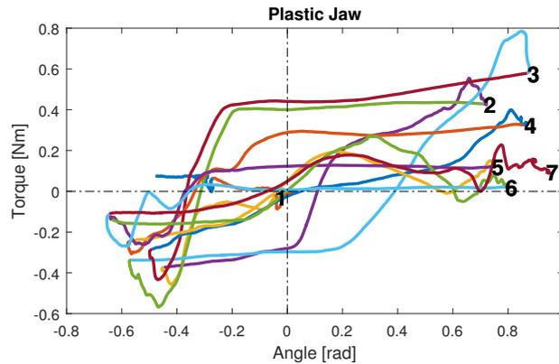
**Figure 5-4:** The torque-angle correlation of the plastic jaw. The shape is different from the one for the pig jaw. However, the change of the slope is similar.
