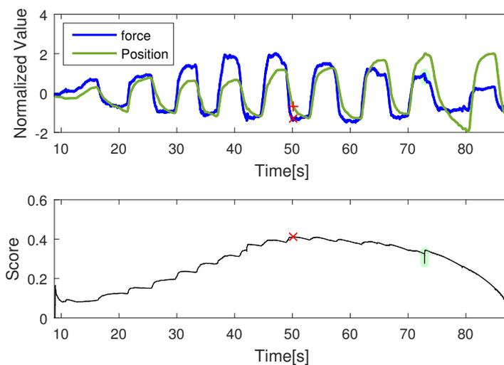
**Figure 4-7:** The result of cracking point detection. The lower part of the figure is the cost function of the change point detection on the force signal. The shade highlight the point the cracking point that is not obvious in the data.
