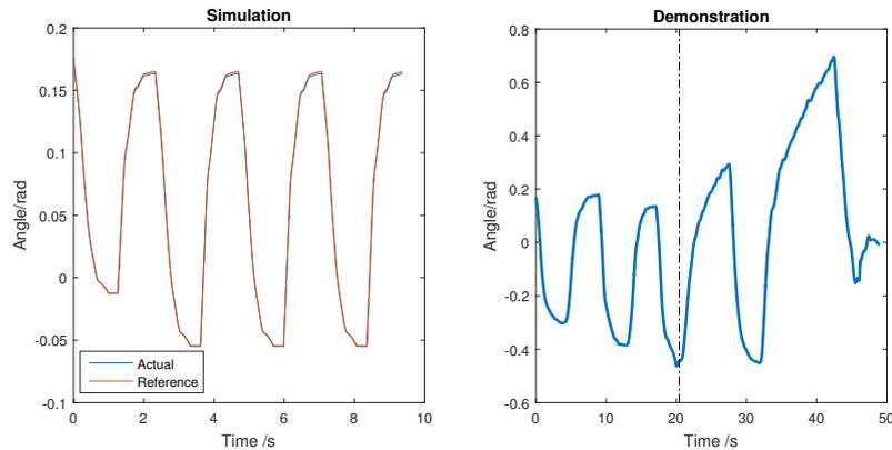
**Figure 8-1:** The comparison between the movement of simulation on the plastic jaw (left) and the demonstration on the pig jaw (right). In the left part, the actual position (blue) tracks the reference (red) successfully. In the right part, the first two iterations of the demonstrations are as same as most lingual and buccal movements. The last two iterations are the ones at the end of tooth extraction when the tooth is very loose.
