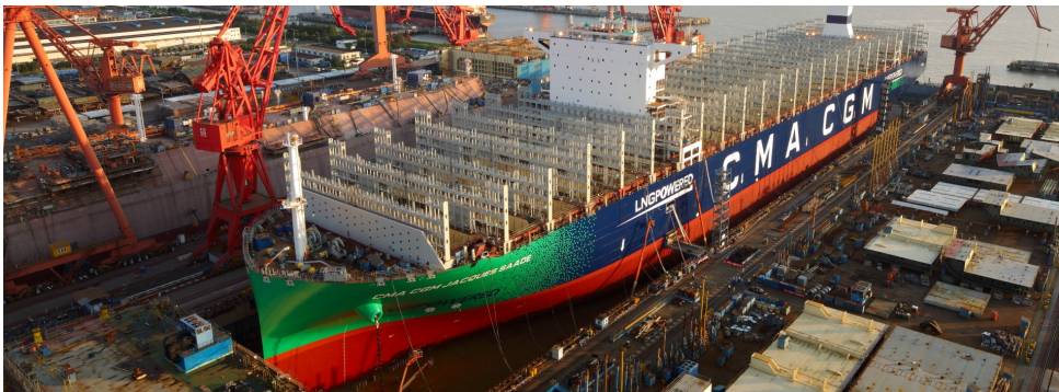
Figure 1.1: LNG-powered CMA CGM Jacques Saade container ship under construction [1]
