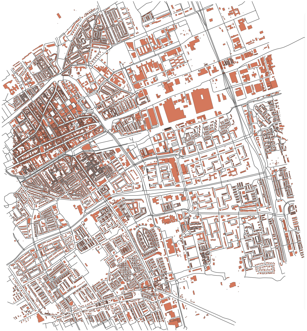
Figure B.3: The BGT building data and NWB road data as it will be input into the road classification algorithm for the city of Delft, Zuid-Holland. The map is turned 90 degrees counter clockwise.
