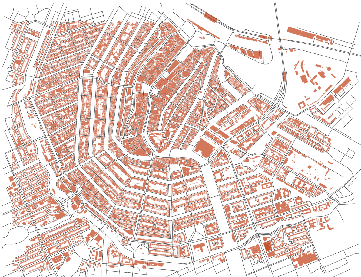
Figure 3.3: The BGT building data and NWB street data as it will be input into the street classification algorithm for the city of Amsterdam.
