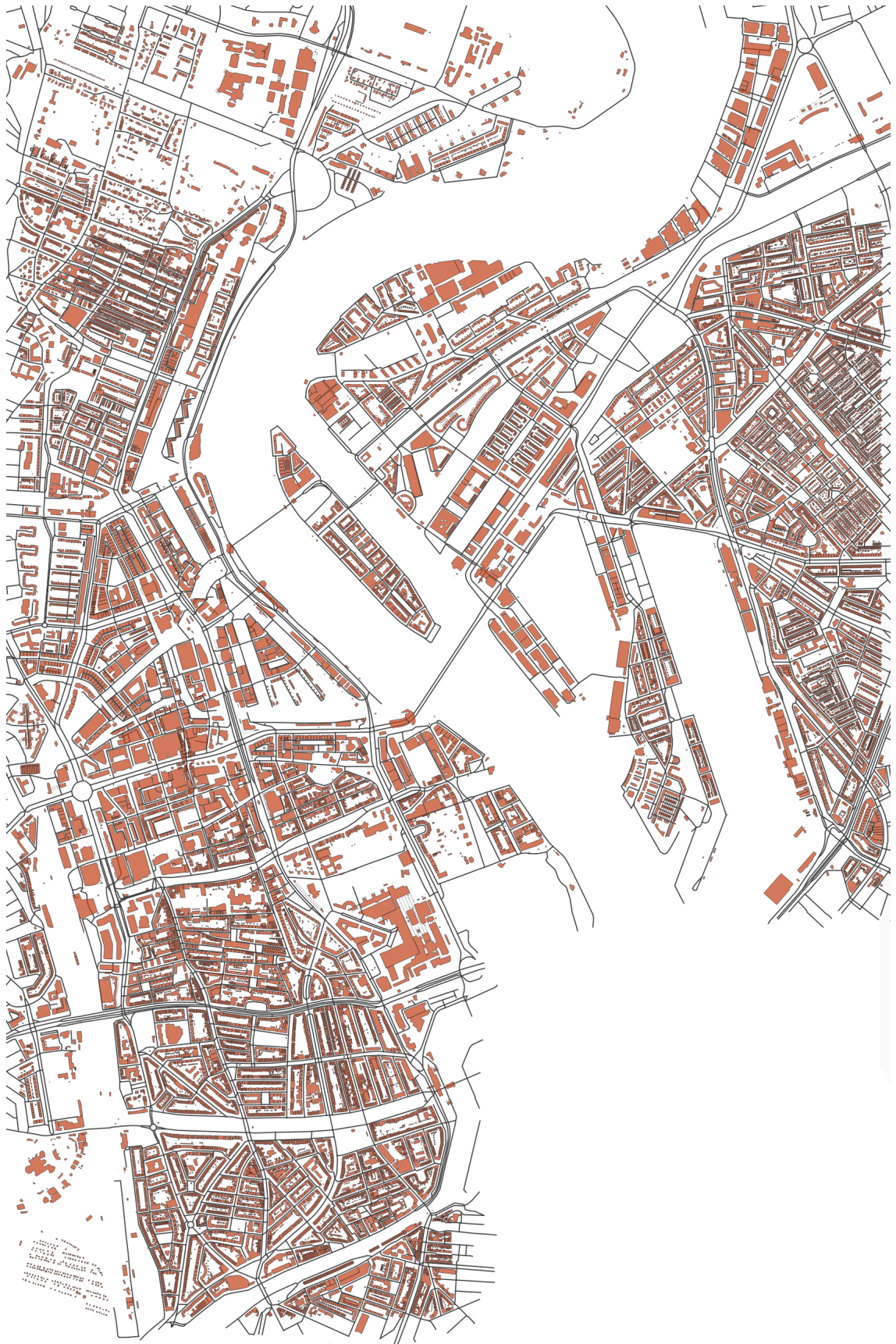
Figure B.1: The BGT building data and NWB road data as it will be input into the road classification algorithm for the city of Rotterdam, Zuid-Holland. The map is turned 90 degrees counter clockwise.
