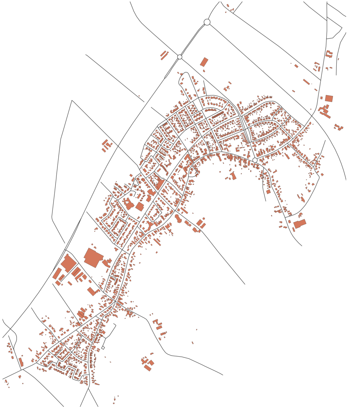
Figure B.7: The BGT building data and NWB road data as it will be input into the road classification algorithm for the town of Posterholt, Limburg. The map is turned 90 degrees counter clockwise.
