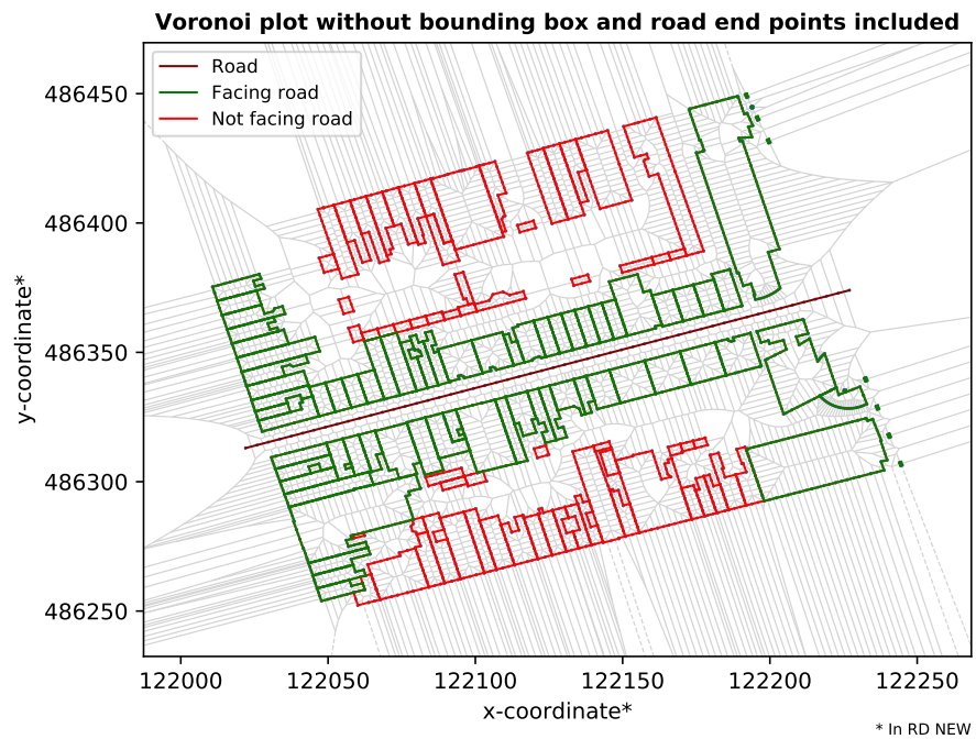
Figure 4.5: A Voronoi diagram created from points making up the street and the buildings. The points represent the generators, and the Voronoi edges are shown in grey. Buildings that do not face the street are detected as facing the street because of the infinite Voronoi cells.
