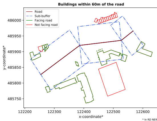
Figure C.3: The image shows the sub buffers created to compute the convex hull of a complex road segment
