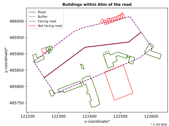
Figure C.4: The image shows the final buffers obtained from the convex hull, after cutting the wrong parts
