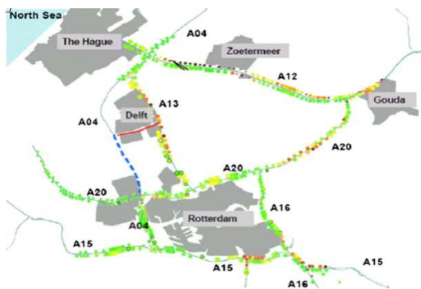
Fig. 6. Map of network of Highways surrounding Delft and traffic density maps, green circles no jams, red circles heavy traffic jams (photo RegioLab-Delft).
