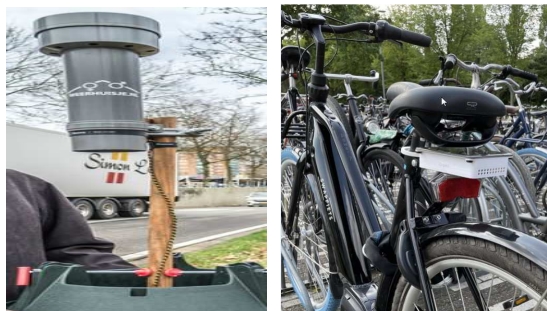
Fig. 1. Fine dust sensor designed by technicians from MLZ. Fig. 2. Mobile fine dust sensor designed by DUT-MIT.
