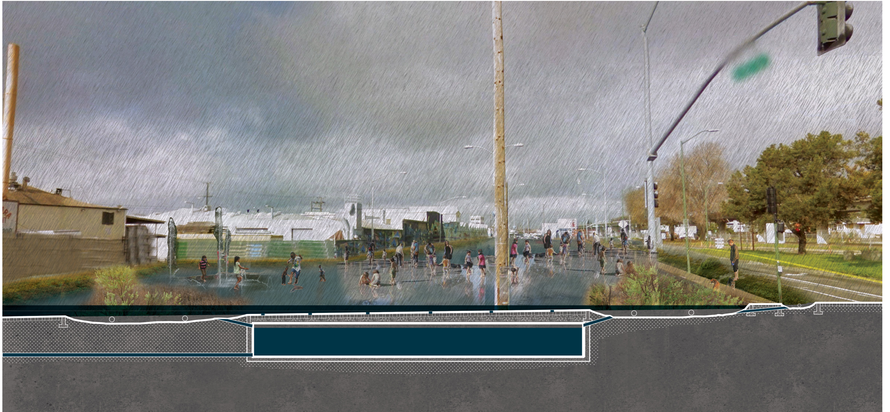
Figure 8.37: Parking facility - wet condition. Illustration : Author
