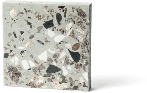
Figure 49. Terrazzo tiles from building waste: the “urban terrazzo” (Source: They Feed Off Buildings).
