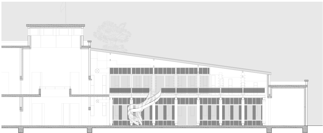
Figure 17. The library: design proposal section, dividing the volume into a gallery with a central stair connecting the ground and first floors (Source: by author).
