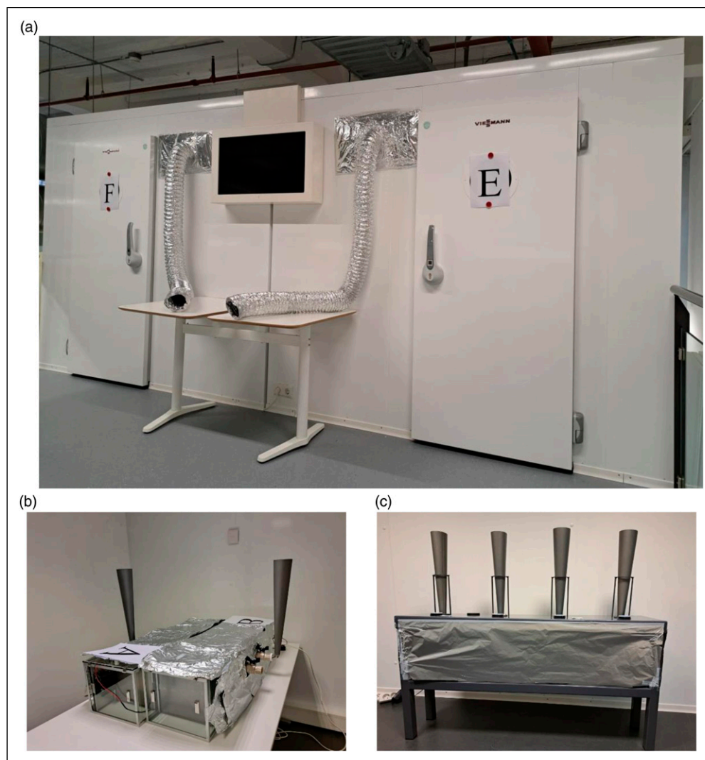
Figure 1. Test environments: (a) test chambers; (b) CLIMPAQs; (c) sniffing table.
