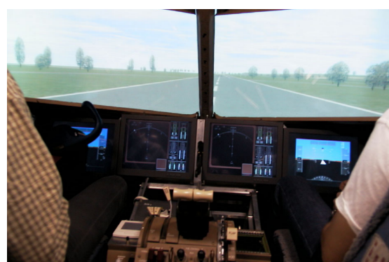
Figure 2.14: Flight deck inside SIMONA. Note yoke on the left and side-stick on the right. Adapted from [41].
