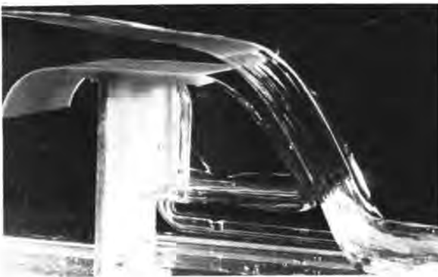
Photo 2. Flow over a round-nose broad-crested weir with rectangular control section.
