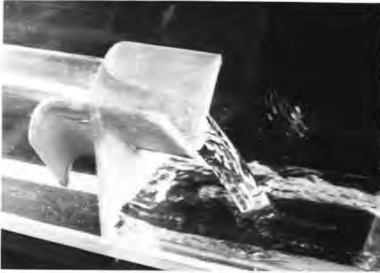
Photo 3. Flow over a broad-crested weir with triangular control section.
