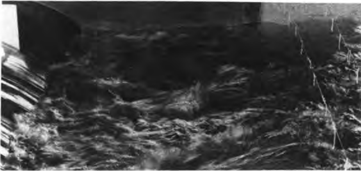
Design B: Tailwater depth is 15% greater than in Design A.
