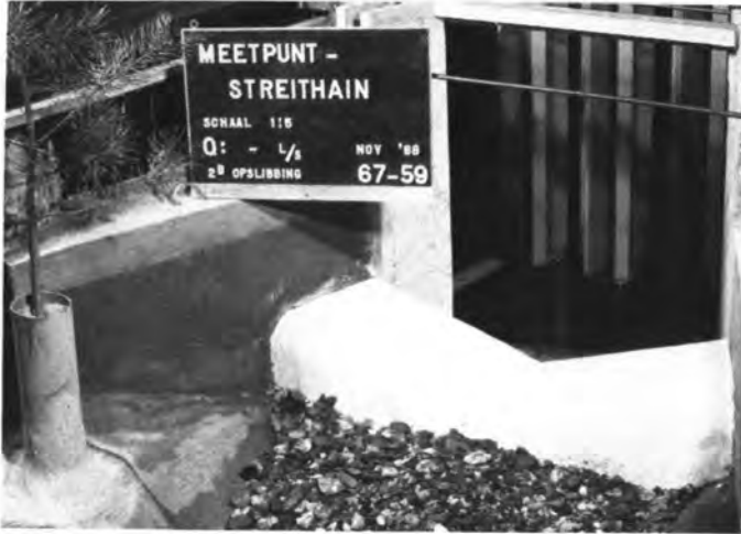
Photo 3. If the limits of application of a measuring structure cannot be fulfilled, laboratory tests can provide a head-discharge curve.
