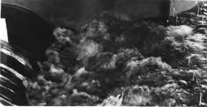
Design A: Tailwater depth calculated by TW/y_2 = 1.1 - Fr_u^2/120 (see Table 2).
