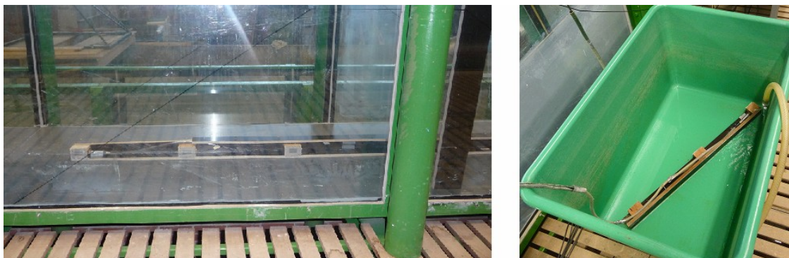
Figure 3.13 – The lodging of sensors in the flume (left) and during calibration (right)
