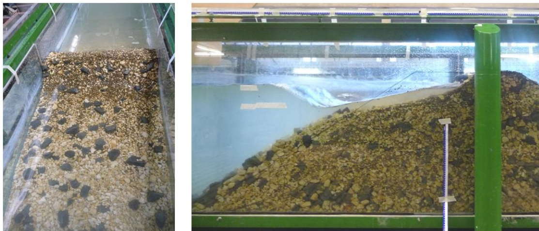
Figure 4.8 – Segregation observed during Test 3
