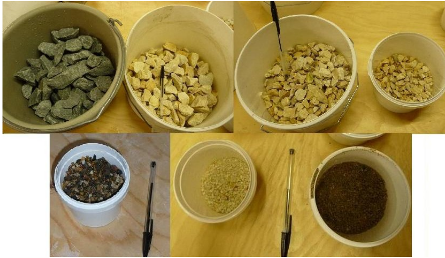
Figure 3.4 – The 7 classes of stones and sand
