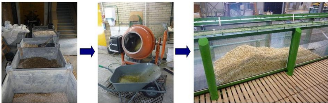
Figure 3.14 – Phases of the construction of the model structure
