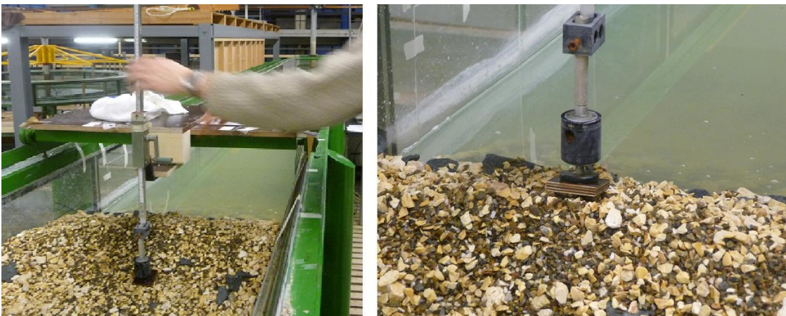
Figure 3.16 – The mechanical device for measuring the cross-shore profile
