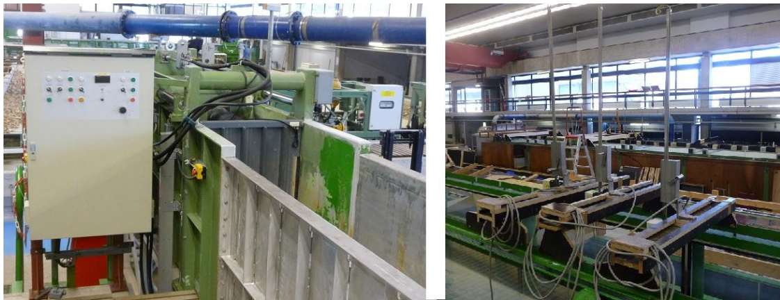
Figure 3.8 – The wave generator and three wave gauges
