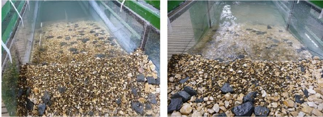
Figure 3.15 – Wall effect observed during Test 3 (left) and Test 5 (right)
