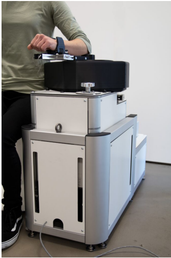
Fig. 1: Overview of the Shoulder Elbow Perturbator (SEP). The participant’s forearm is attached to the lever arm, while the elbow joint is aligned with the motor rotation axis to enable controlled perturbations. Source: https://hankamprehab.nl/de-schouder-elleboog-perturbator-sep/
