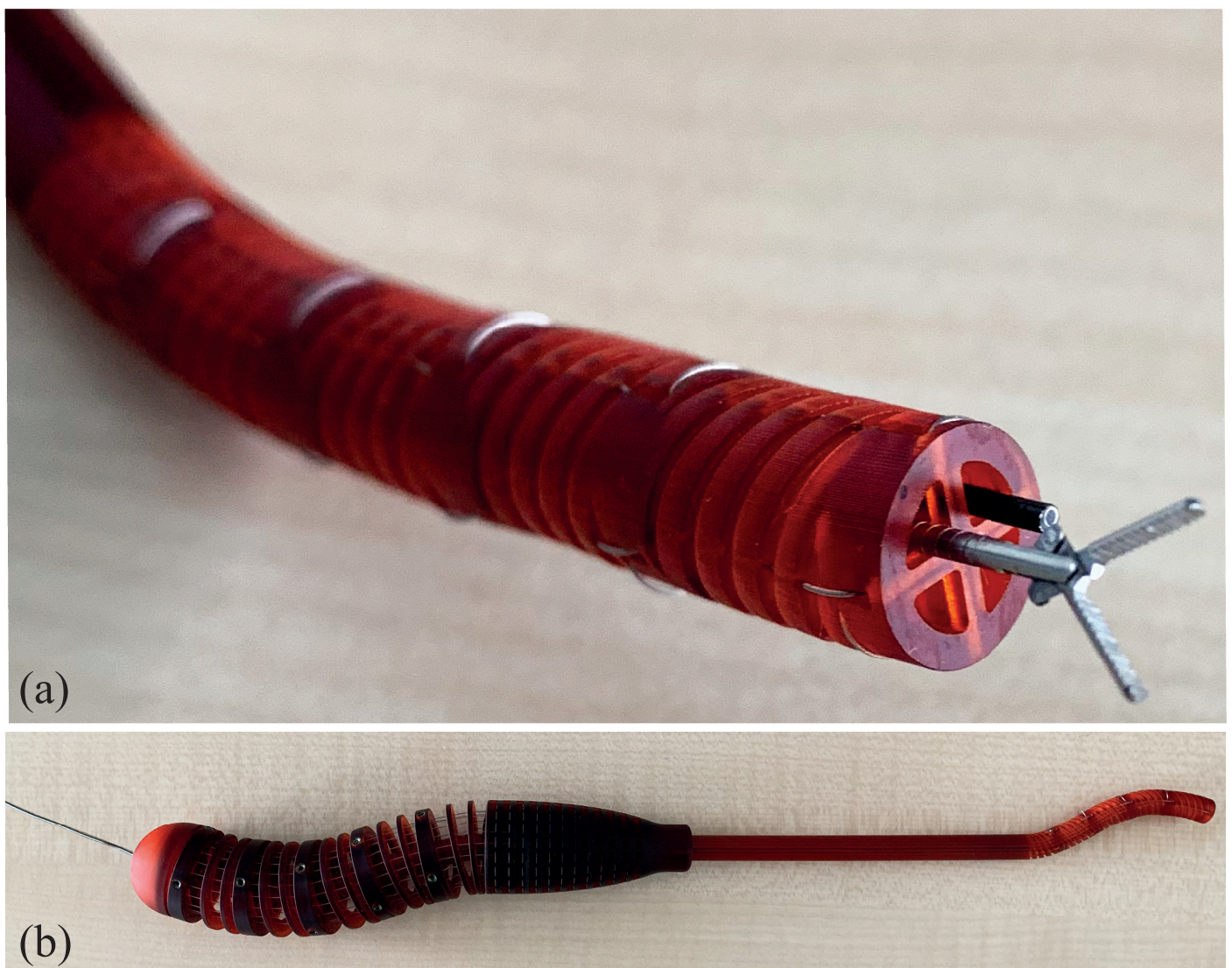
Fig 8. Pictures of the HelicoFlex prototype. (a) close-up of the compliant shaft of the HelicoFlex with a flexible biopsy forceps in one lumen and a flexible fiber optics endoscope in the second; (b) bendable metal rod inserted into one of the lumens to create a certain shape in the compliant shaft and keep it in position.
