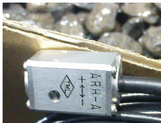
Fig. 2.29: Accelerometer before the installation on the ELASTOCOAST revetment
