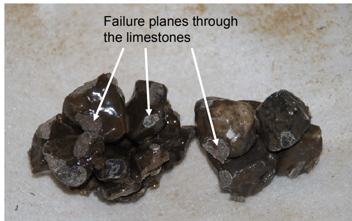
Fig. 8.7: Failure through limestones (Oumeraci et al, 2009a)
