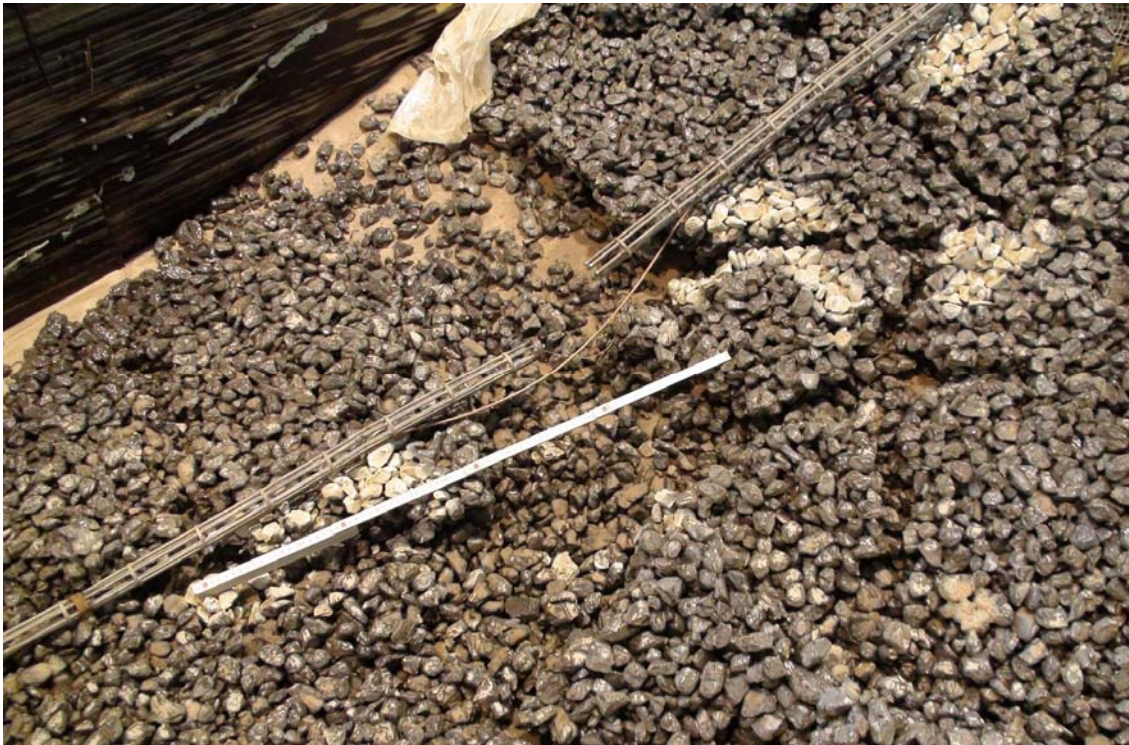
(a) Unexpected breakage in several blocks
