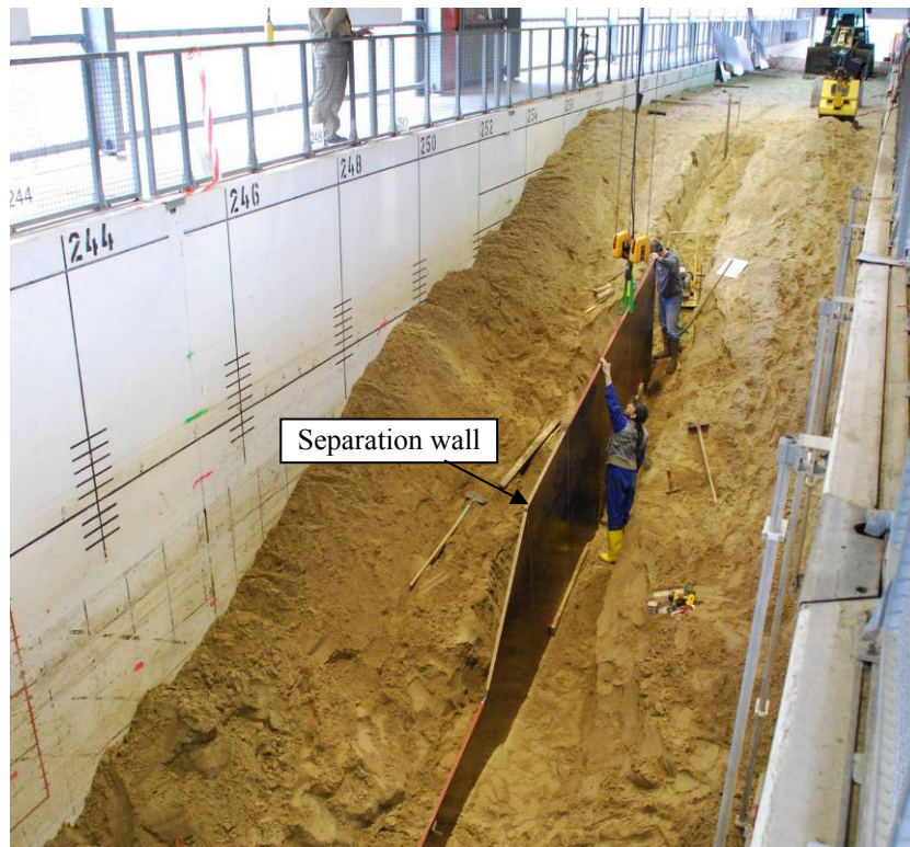
(a) Positioning the wall
