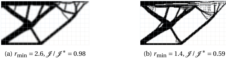
Figure 7.17: Optimized designs for cantilever beam subjected to distributed load (as in Fig. 7.1) for two different filter radii. The domain is discretized using 20 \times 10 finite elements with shape functions of polynomial degree 6 and 8 \times 8 design voxels per element.
