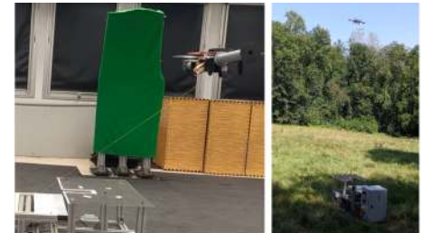
The experimental setup : The ground station and the tethered hybrid Quadcopter/Magnus-effect wing UAV.
