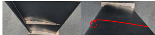
Rigid LEI airfoil model representing an extruded mid-span section of the TU Delft V3 kite; pressure side (left) and suction side (right).
