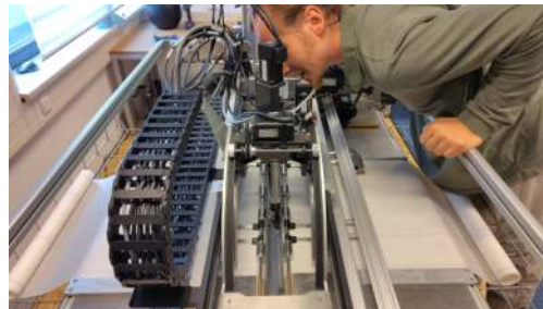
Sean Carslaw Tricot hunching over the wavemaker01, watching as the tapes are placed and welded between the membranes.
