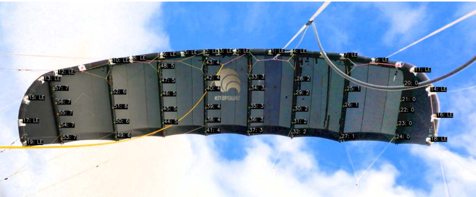
Kitepower's V3 kite with marker indexing on the wing during flight. The distinction between the leading-edge (LE) markers and the strut markers is indicated, with the strut markers numbered from 0 to 7. Some markers remain unidentified, either because they do not pass the detection filters or because they are occluded in either of the camera views. Pim J. Haanen: In-flight experimental measurements of large-scale deformations on a leading-edge inflatable kite using stereoscopic photogrammetry and UWB modules. MSc Thesis, Delft University of Technology, the Netherlands (2026). edu.nl/ke9kq
