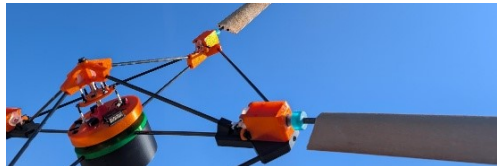
Figure 2: Rotary AWE system developed by someAWE.
