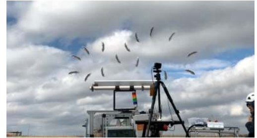
Images superimposed to depict the Figure-8 flight path of the AWE kite during Phase 2 test in March 2023
