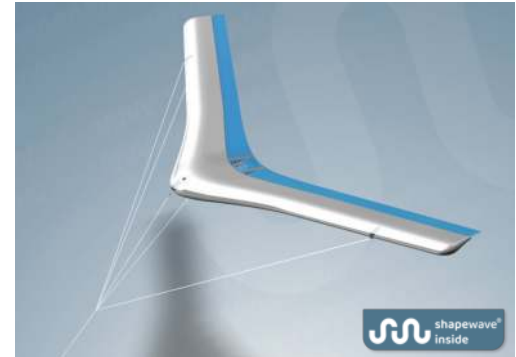
CAD screen shot of the 5 m span Toyota Mothership/TRINA test wing 1 , with an inflatable main section and a stitched rip-stop trailing edge, with triple functionality: (1) housing for electronics; (2) light-weighting and aerodynamic improvement; (3) integrated control surfaces.
