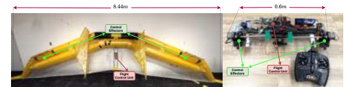
Fig. 1: Overview of proposed KITELab iron bird. The image on the left shows a fully inflated tethered-wing system with bio-inspired flaps as a control effector. On the right side, we have our KITELab testbed with a compact placement of the flight control unit and the control effectors.
