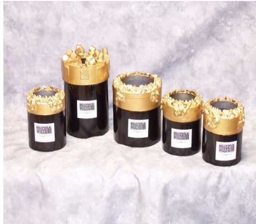
Figure 2.2: Core drill bits (manufacturer Ceramco Pty Ltd) used to obtain cores of a formation.
