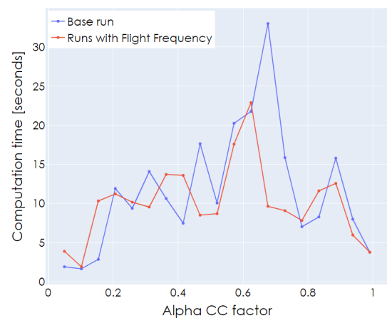
Figure 21: Computational time of the base case and the case with flight frequency consideration per run case ( \alpha_{CC} )
