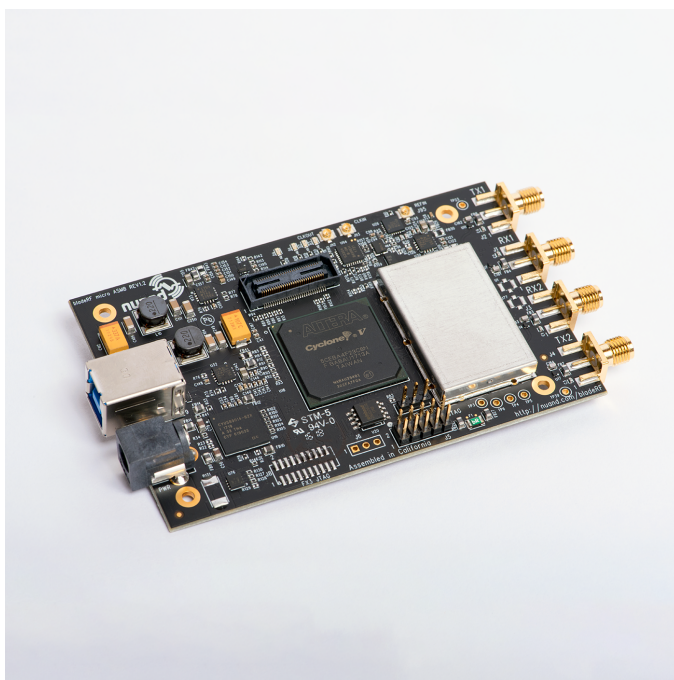
Figure 7.3: The Software Defined Radio used [image from nuand.com]
