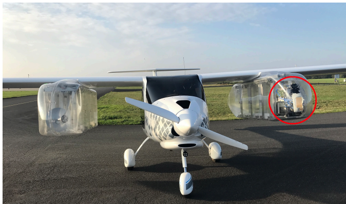
Figure 5.11: The test aircraft, with the radar in the port freight container
