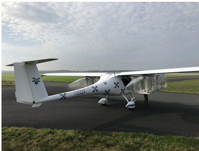
Figure 3.22: The aircraft used for detection, with the cargo boxes under the wings
