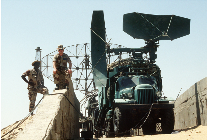
Figure 1.4: Precision Approach Radar hardware, pictured in 1985
