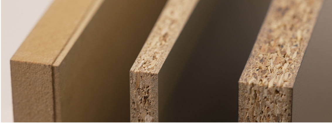
Fig. 5.6 Close-up of flax particle board (Unilin, n.d.)
