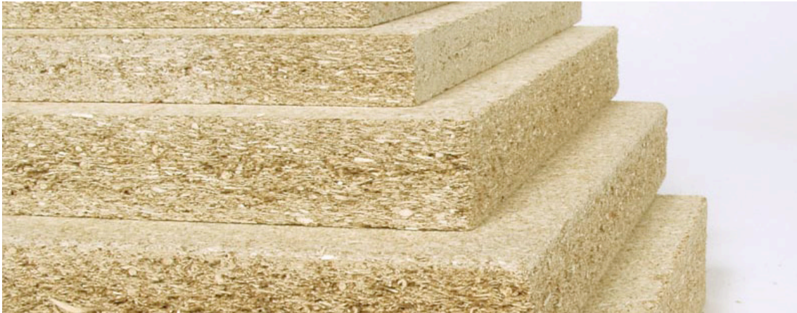
Fig. 5.14 Close-up of particle board with miscanthus (Linex, n.d.)
