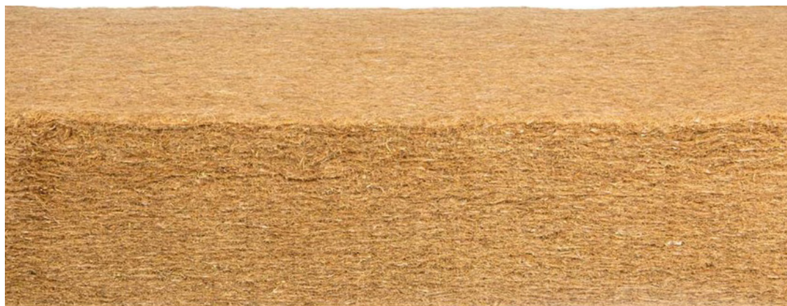
Fig. 5.11 Close-up of hemp insulation (Hempflax, n.d.)
