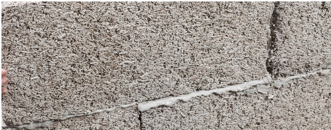
Fig. 5.12 Close-up of hempcrete (Isohemp, n.d.)
