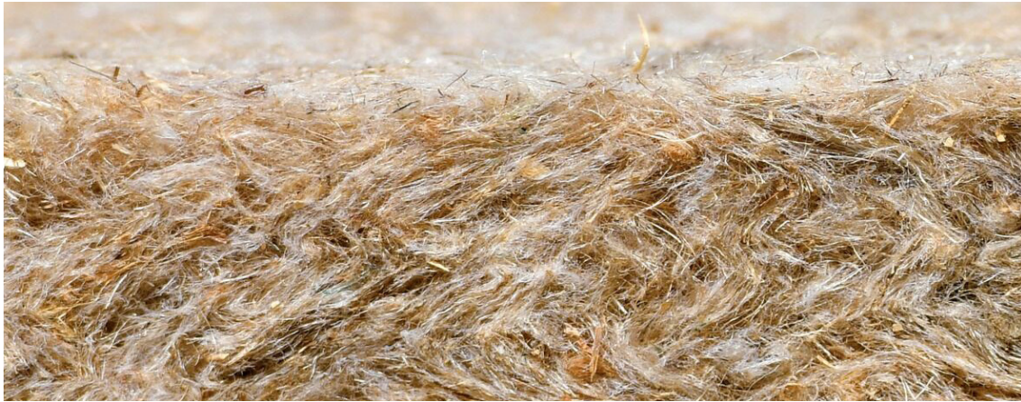
Fig. 5.8 Close-up of flax insulation (Isovlas, n.d.)
