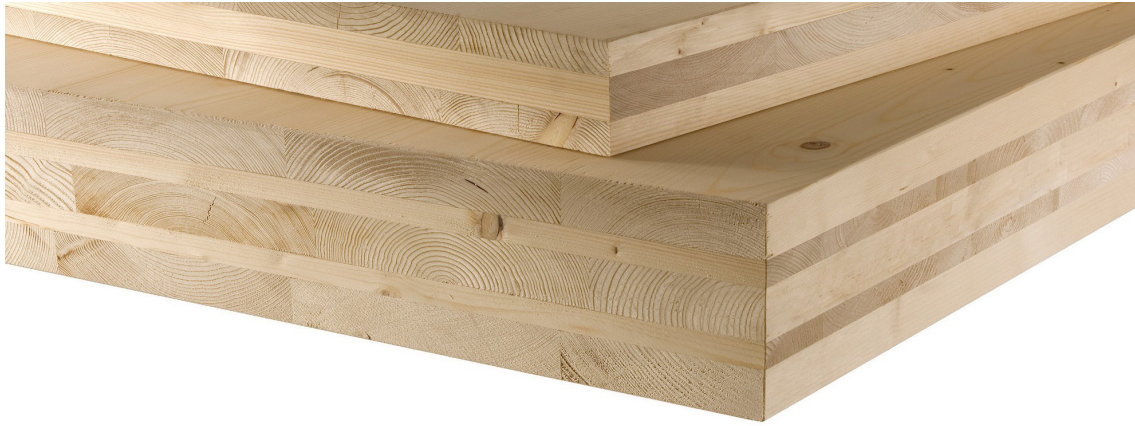
Fig. 5.4 Close-up of cross laminated timber (Stora Enso, n.d.)
