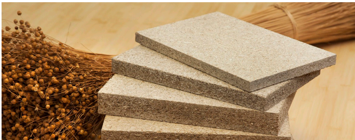
Fig. 5.10 Close-up of flax particle board (Linex, n.d.)
