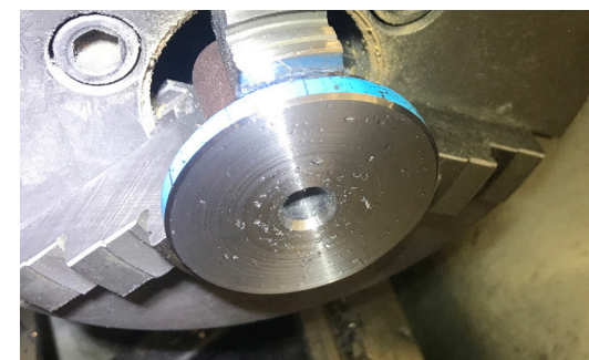
Step 4. Product is turned around; hole is drilled (10mm)
