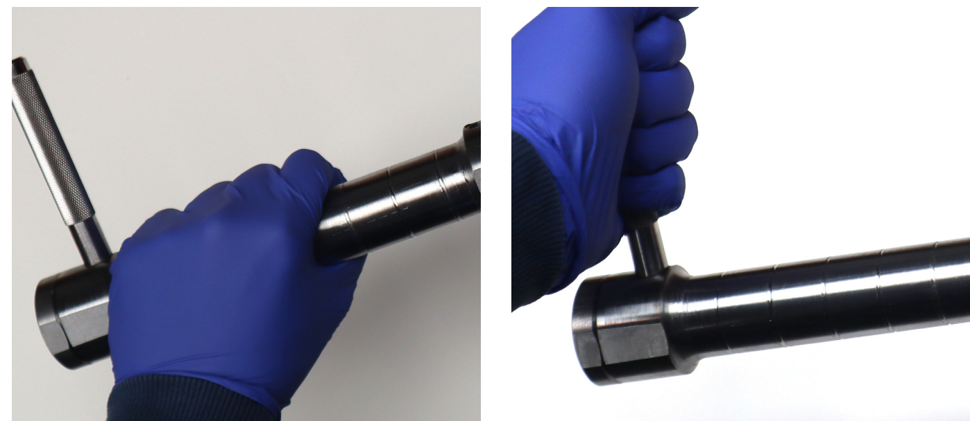
Figure 4.9. Powergrip onto the mainbody and gripping on the installed steering handle
