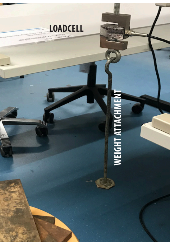
(15.2) Scaime ZFA 500 kg Loadcell loaded in tension to calibrate with weight attachment (Left corner plates of 10 kg are used as weight)
