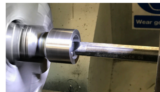
Step 3. Milling hole to 28 mm, to accommodate M30 tap
