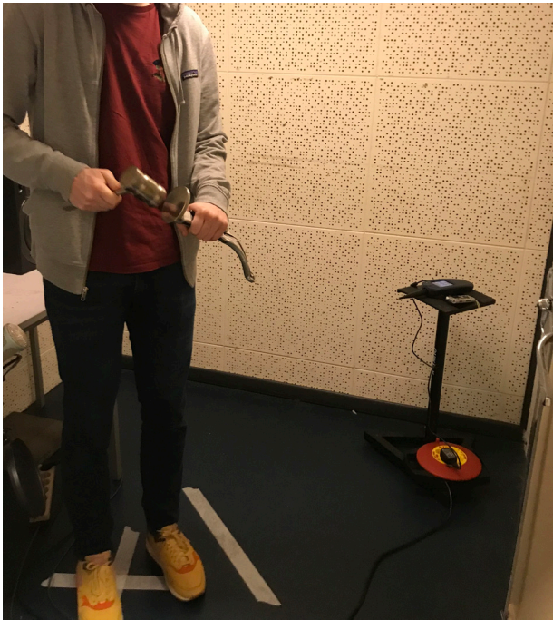
Figure 4.17. Test set-up in sound studio, using current mallet (*studio-door was closed during testing*)
