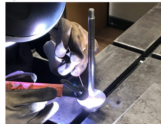
Step 6. Rod is welded into the drilled hole
