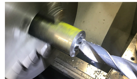
Step 2. Hole is drilled of 26 mm diameter
