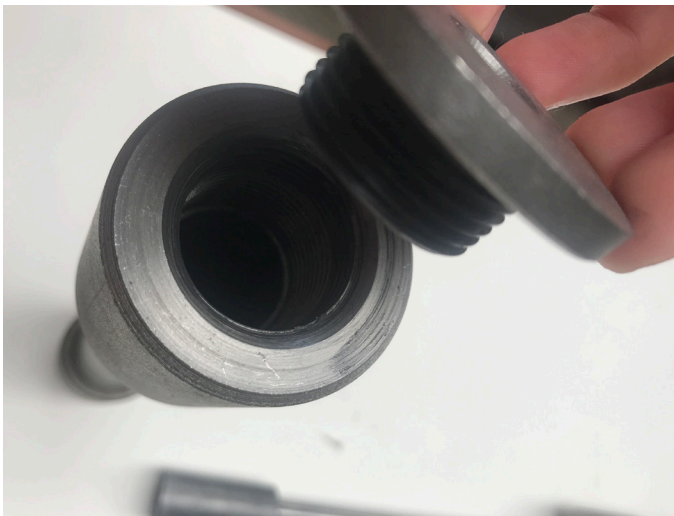
(14.5) Threaded connection on top of main body and guider cap (M30x2)
