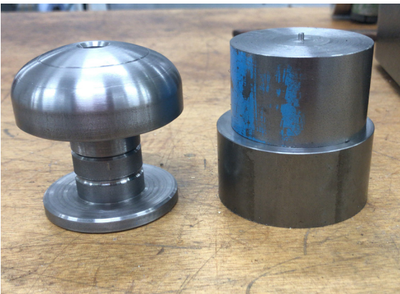
Figure 4.13. The final product vs. Raw material (difference in material is estimated to be around 50%)
