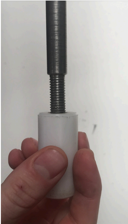
Step 2: Piston onto Driving rod
