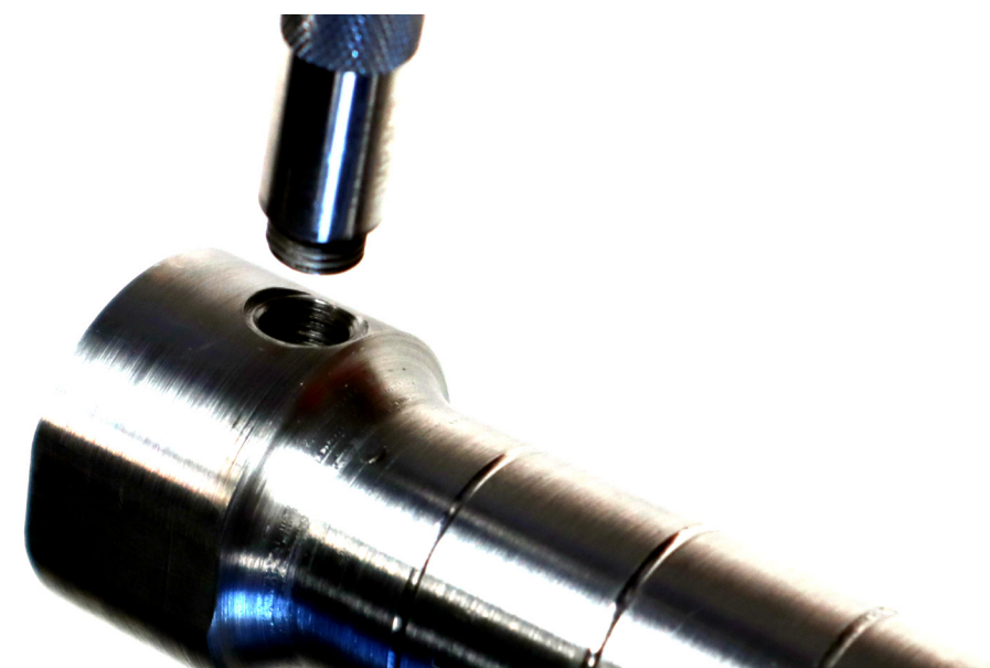
Figure 4.8. Threaded holes allow for connection of steering handle
