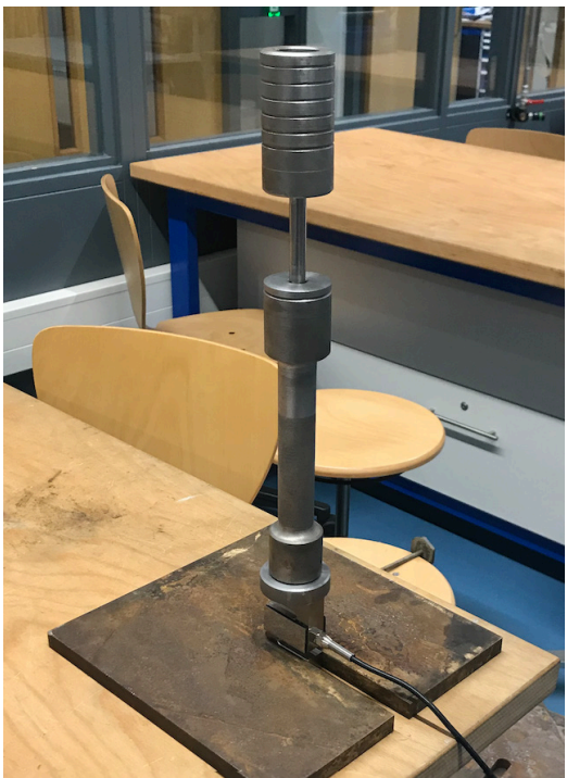
(15.4) Scaime ZFA 500 kg with strikeplate on top
