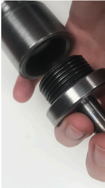
Step 6: Screwing modular attachment onto the DriveFit main body
