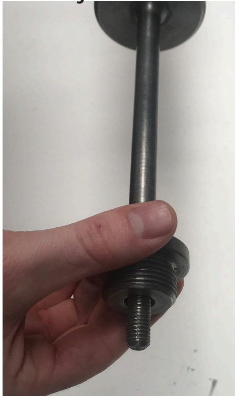
Step 1: Guidercap over Driving rod
