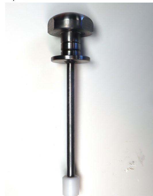
Figure 3.72. Result fully fabricated Driveshaft with Piston.
