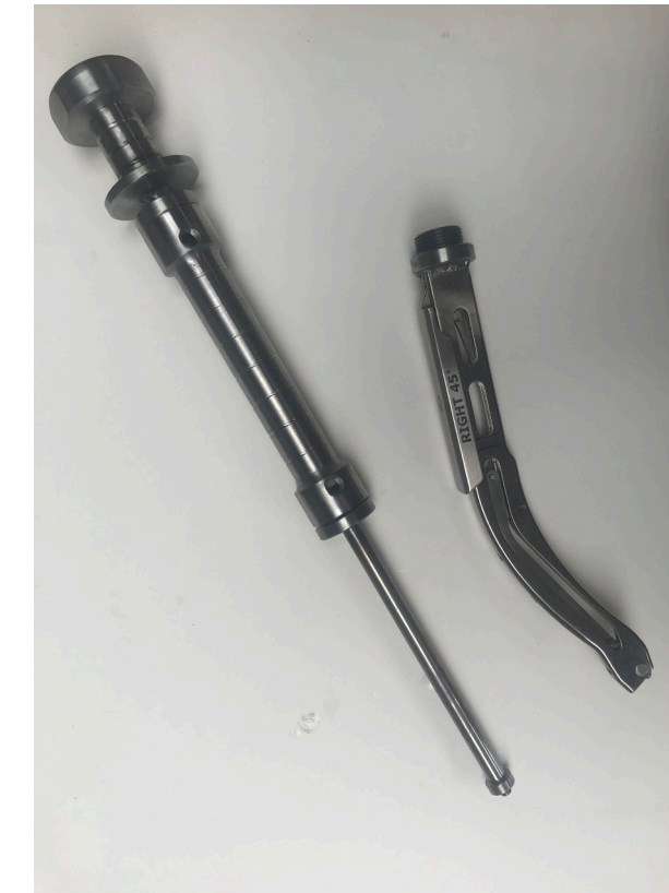
Figure 4.31. How DriveFit will be assembled before surgery with Acetabular cup (Left); Broaching adaptor (right)
