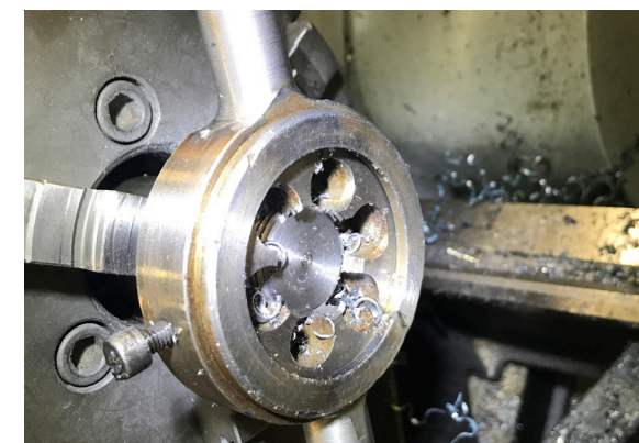
Step 3. Thread cutter; Die M30x2 is made
