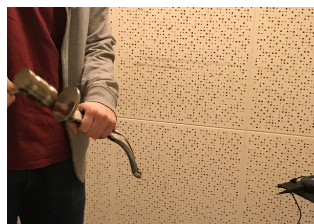
Figure 3.25. Test set-up: Striking broaching handle with surgical mallet
