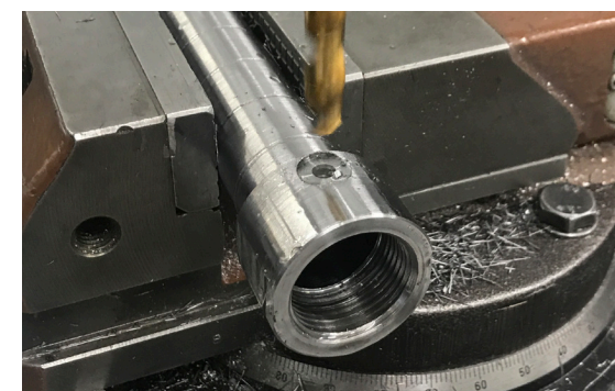
Step 5. Milled flat surface and drilling hole to accommodate tap for steering handle attachment
