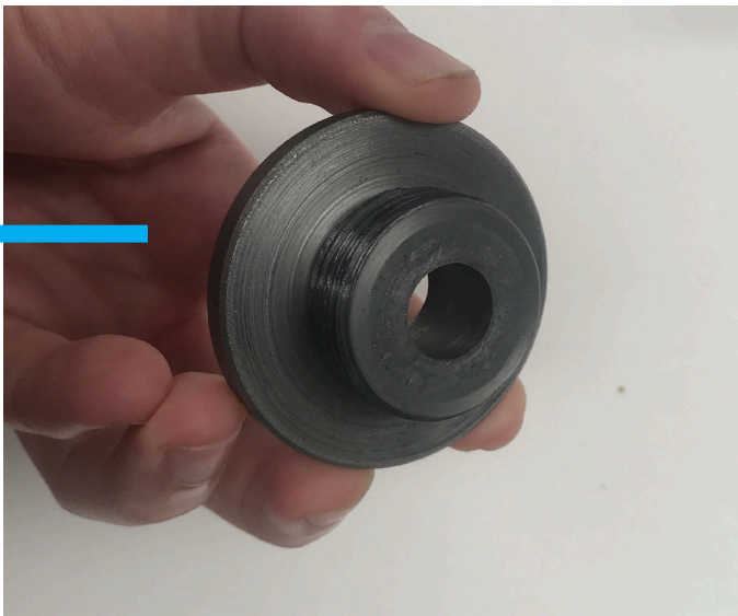
(14.7) Guider cap with hole for driving rod; connected to the top of the main body
