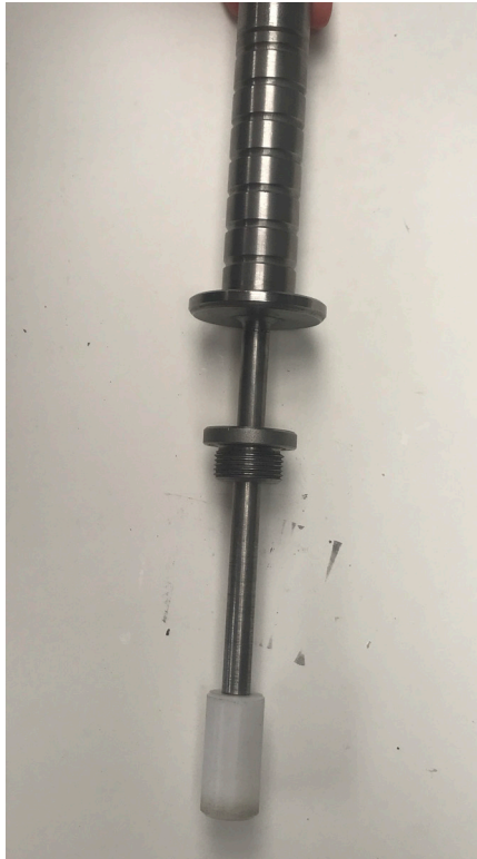
Step 3: Full assembled handle + Driving rod
