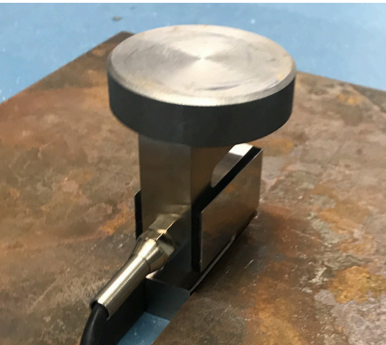
(15.3) Scaime ZFA 500 kg with strikeplate on top
