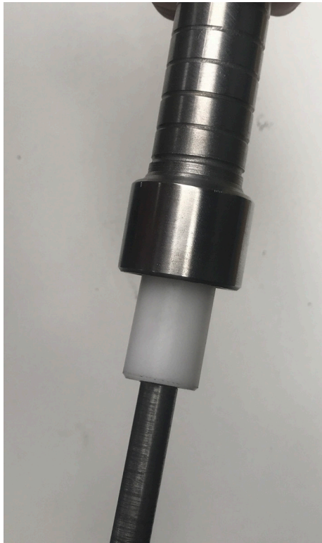
Step 4: Pushing driving rod into main body
