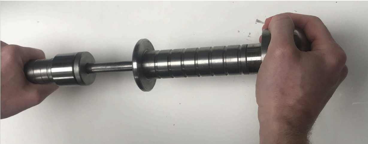
(18.8) New modular handle; Impacts and extraction with added weight
