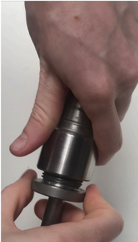
Step 5: Screwing guider cap onto Main body
