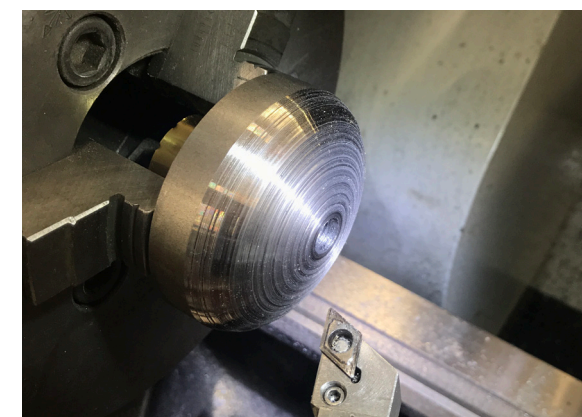
Step 1. Done on Lathe not CNC machine when prototyping; hard to make the half dome shape
