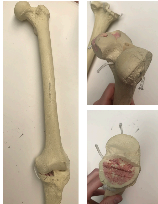
(21.1) Left leg human replica sawbone (Left); Rightside top is Femur knee side and below Tiba knee side, used for impaction.
