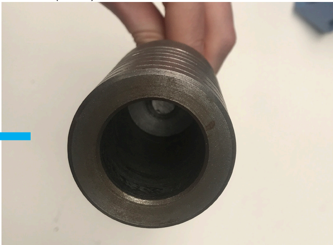
(14.7) Hollow handle as weight reduction (otherwise it was too heavy)
