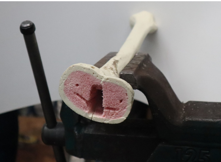
Figure 4.26. Set-up of bone in the vise; Looking at the Tibia plateau Photo taken after broaching the sawbone
