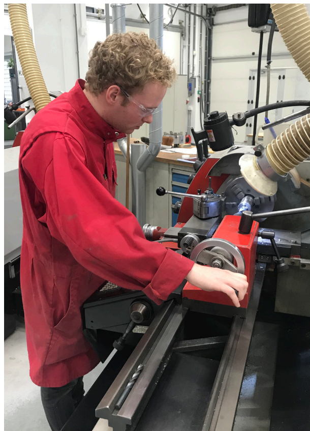
Figure 3.15. Prototype 1, being made at PMB. (Fully produced on lathe)
