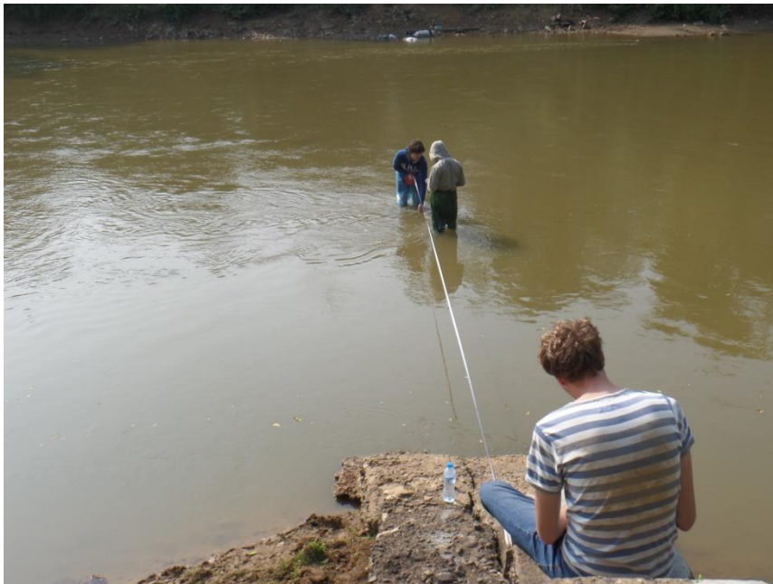
Figure 40 Velocity area method at measurement location
