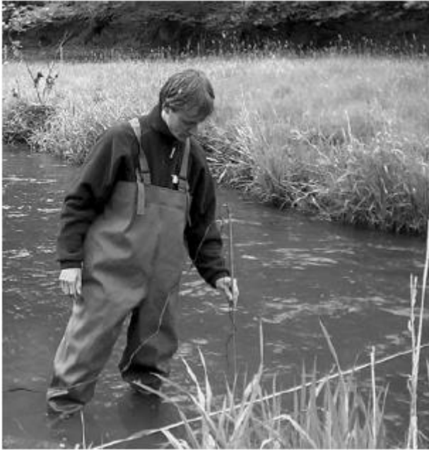
Figure 42 Use the propeller current meter 36
