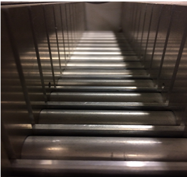
Figure 18. Picture of the position sensitive detector consisting out of 16 helium tubes.
