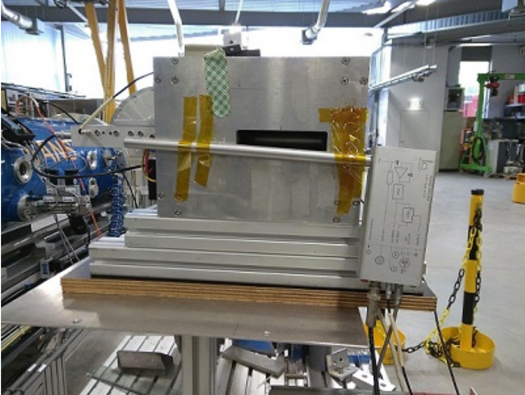
Figure 17. Picture of a 1cm helium tube taped to a beamstop.
