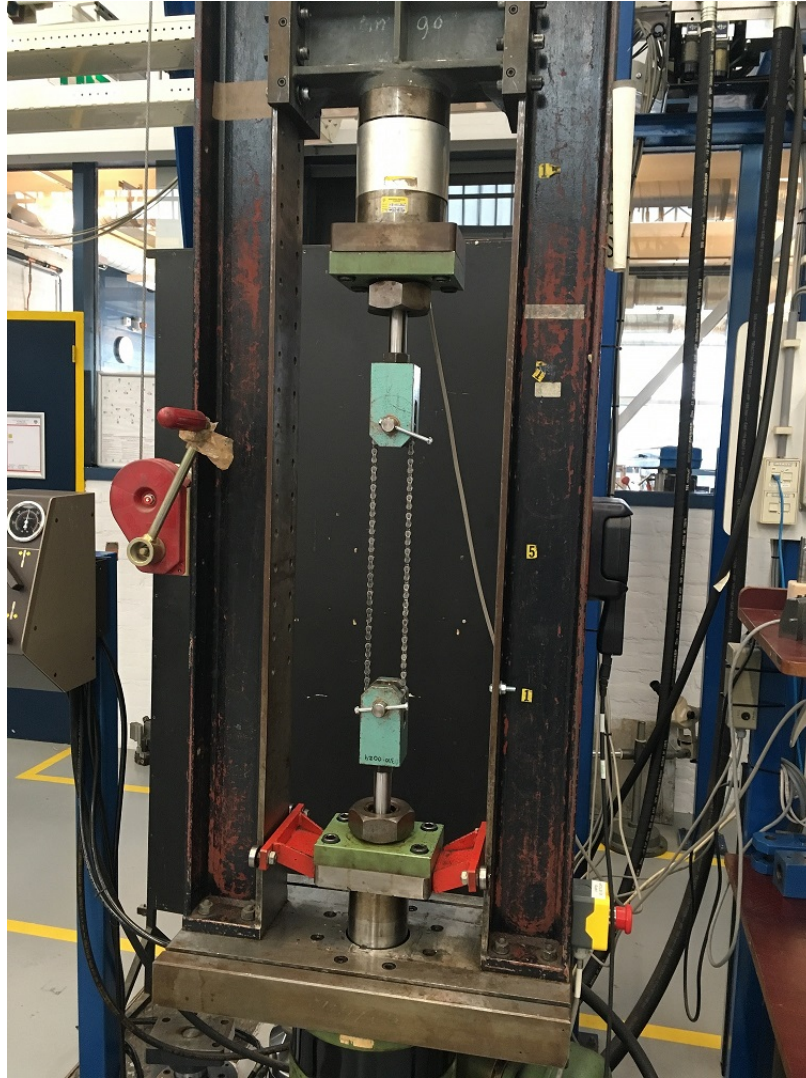
Fig. 5 Example bicycle chain in test machine.
