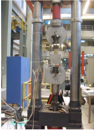
Figure 42: The bamboo specimens tested in a hydraulic testing machine.
