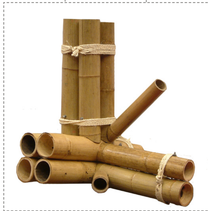
Figure 47: building the bamboo prototype scale 1:1
