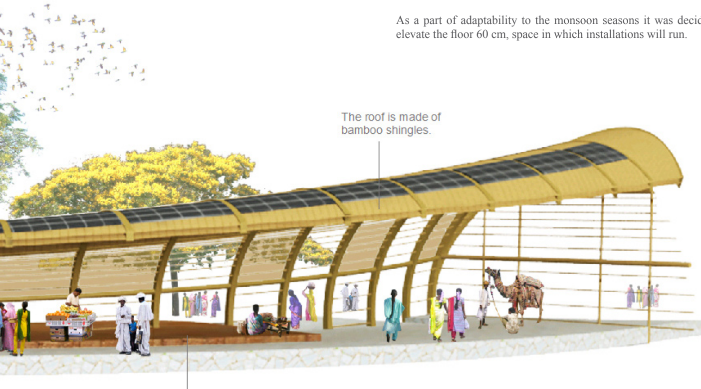
Figure 25: Section of the Communal Centre.
