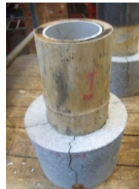
Figure 43: Cracks of the concrete due to concentration of stresses.
