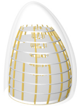
Rammed earth skin is completely detached from interior structure.
