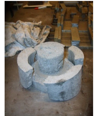
Figure 43: Cracks of the concrete due to concentration of stresses.
