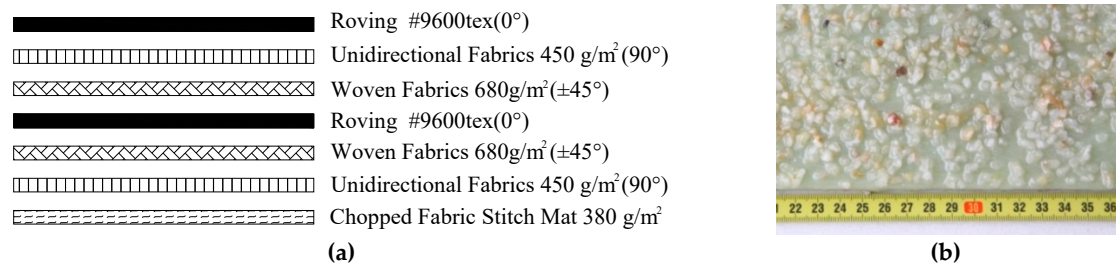
Figure 1. Sand-coated glass fiber-reinforced polymer (GFRP) plate. (a): Layers of pultruded GFRP plate; (b): Sand-coated treatment surface, (unit: cm).
