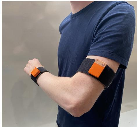
**Figure 1-3:** Two wearable IMUs from the Xsens wireless system used in this thesis, attached to a human subject's arm.
