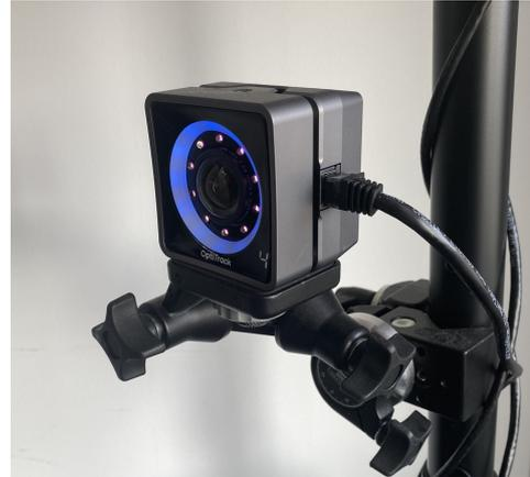
(b) An infrared camera for motion capture from the OptiTrack motion capture system that was used in this thesis.
