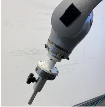
(a) The force/torque sensor and the handle as they were attached to the robot.
