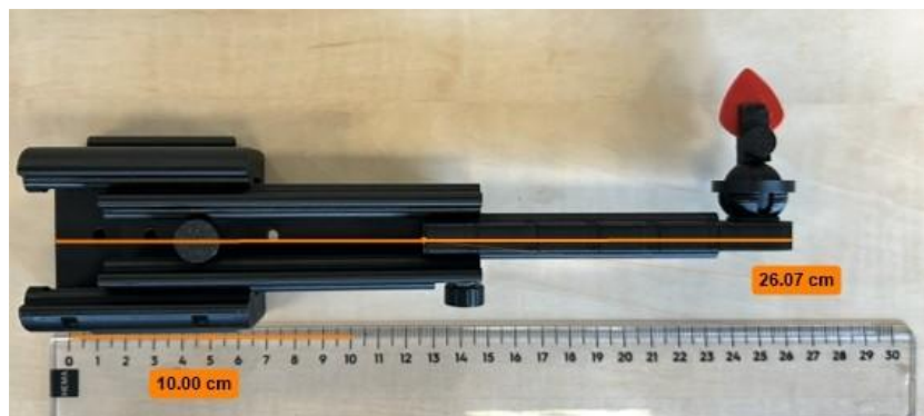
Fig. 20. Length validation on extended model
