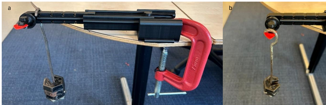
Fig. 24. Model under load with 26 cm: (a) distal part & (b) on plectrum
