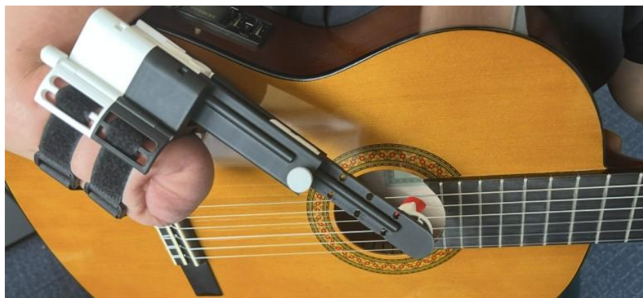
Fig. 14. Final model attached to user's residual limb and elbow resting above the guitar.
