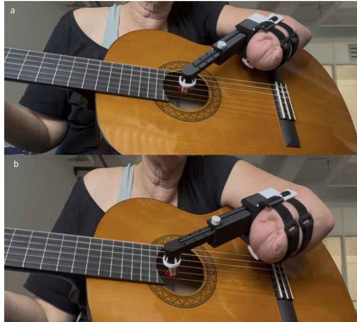
Fig. 27. Device functionality test results of Participant 1: (a) playing the notes with elbow placed on top of guitar & (b) elbow moving freely
