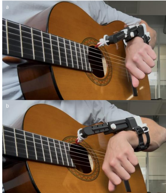
Fig. 28. Device functionality test results of Participant 7: (a) playing the notes with elbow placed on top of guitar & (b) elbow moving freely
