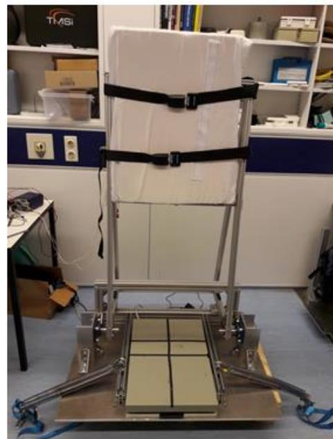
**Figure 14:** Photo of rack 3 with force plate and rail trolley system
