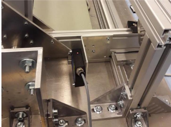
**Figure 7:** Laser distance sensor attached to the backboard
