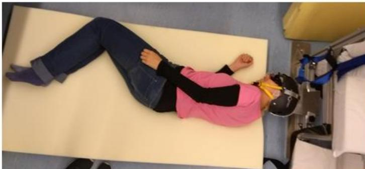
helmet is clamped to the horizontal profile to support head-straight position.
