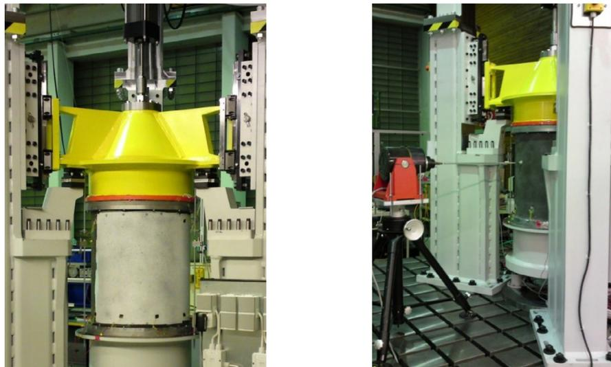
(a) Cylinder ZD28 positioned in the test facility. (b) Shaker with rod coupled at cylinder ZD28.
