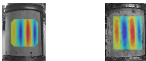
Fig. 10. First unloaded vibration mode of ZD28 and ZD29.
