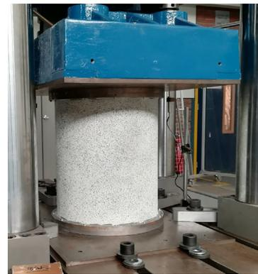
Fig. 11. Cylinder ZD27 positioned in the TU Delft test machine.
