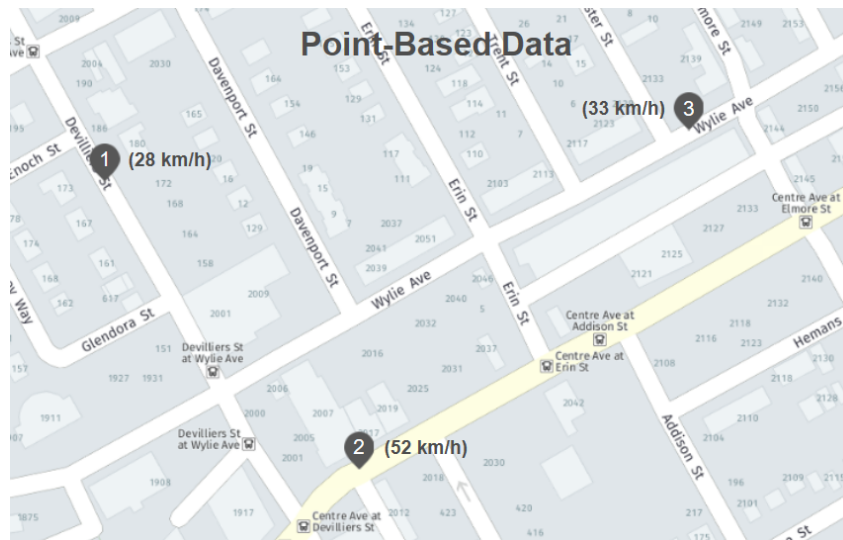
Figure 2.4: Example of GPS data points used to train the speeds with point-based data. Also the driven speed in km/h is included to each GPS point.
