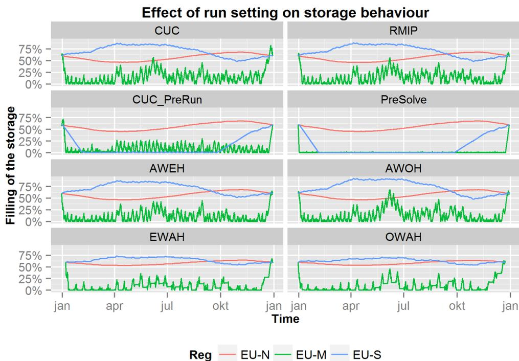
Figure 4-12: Effect of model type on hydro storage levels
