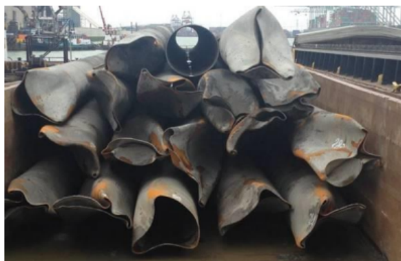
Figure 3.4: Pile tip damage from Rotterdam harbour (Broos et al., 2017; Randolph, 2021).
