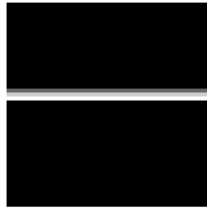
(a) Geometry with small section of gradient with \rho = 0 ; \rho = 0.2 ; \rho = 0.6 ; \rho = 1 from bottom to top, all other elements have \rho = 1
