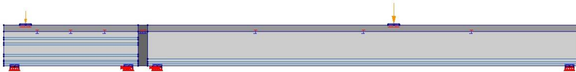
Figure 3.7 Models 1.1-1.2 with linear elastic material properties and varying interface material models
