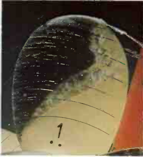
PLATE 7.5. CAVITATION OBSERVATIONS IN THE CAVITATION TUNNEL ON PROPELLER S AT J=0.4 . ( Re_n=1.78 \times 10^6 , \sigma_n=1.3 ).
