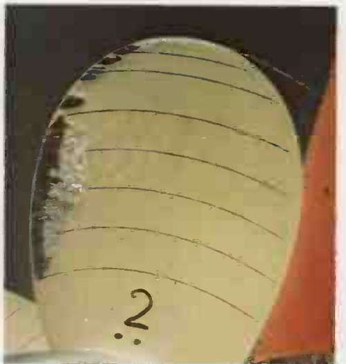
PLATE 7.6. CAVITATION OBSERVATIONS IN THE CAVITATION TUNNEL ON PROPELLER S AT J=0.4 . ( Re_n=1.36 \times 10^6 , \sigma_n=2.2 ).
