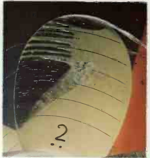
PLATE 7.5. CAVITATION OBSERVATIONS IN THE CAVITATION TUNNEL ON PROPELLER S AT J=0.4 . ( Re_n=1.78 \times 10^6 , \sigma_n=1.3 ).
