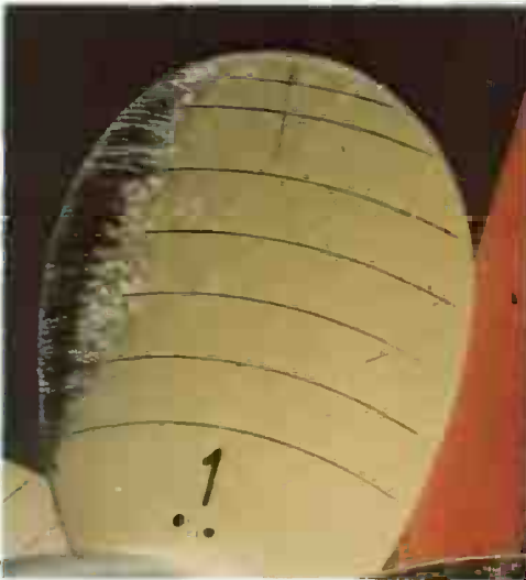
PLATE 7.6. CAVITATION OBSERVATIONS IN THE CAVITATION TUNNEL ON PROPELLER S AT J=0.4 . ( Re_n=1.36 \times 10^6 , \sigma_n=2.2 ).
