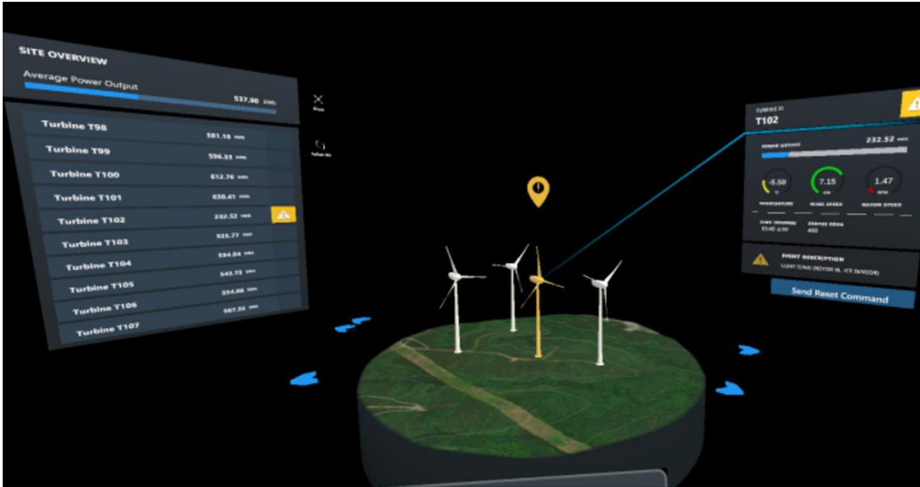
Figure 39: An example of a digital twin application for a windfarm built in Unity (source: Unity & 4Subsea)
