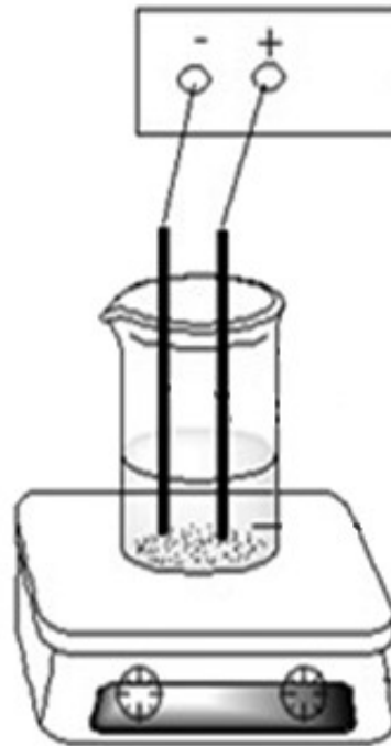
Figure 1.1: Schematic representation of an electrocoagulation reactor with one anode and cathode [97]
