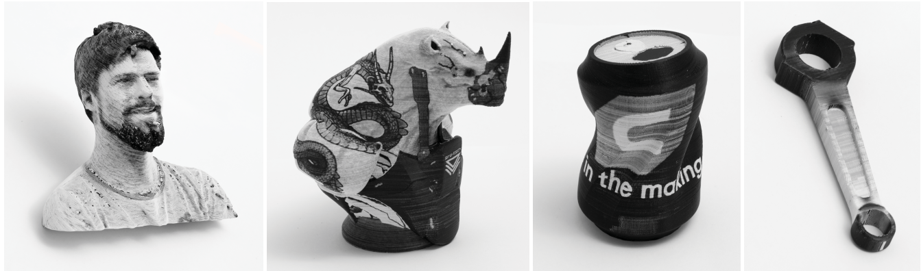
Figure 1: 3D prints obtained by applying vertical and diagonal hatching on a 14 cm 3D scan, a 15 cm artistic figurine, a full size soda can with textual information, and the result of a stress analysis performed on a 16 cm connecting rod of a piston engine.
