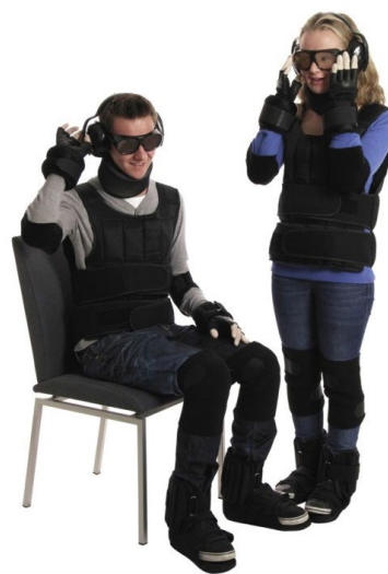
Image 38: GERontologic Test suit "GERT" used by designers to simulate older age to gain sympathy for elderly users (Produkt + Projekt Wolfgang Moll, n.d.).
