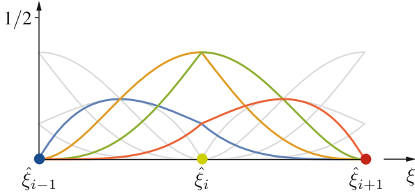
Fig. 3 Global basis for piecewise linear blending function with q_w = 1 and local cubic Bézier basis with q_p = 3 restricted to the chart domain \hat{\Omega}_i = [\hat{\xi}_{i-1}, \hat{\xi}_{i+1}]
