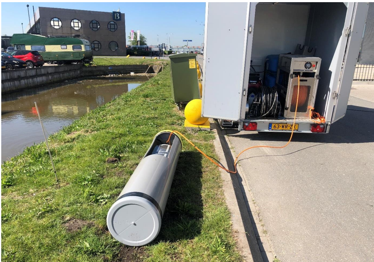
Figure 7: Test set-up A: PVC pipe above the surface
