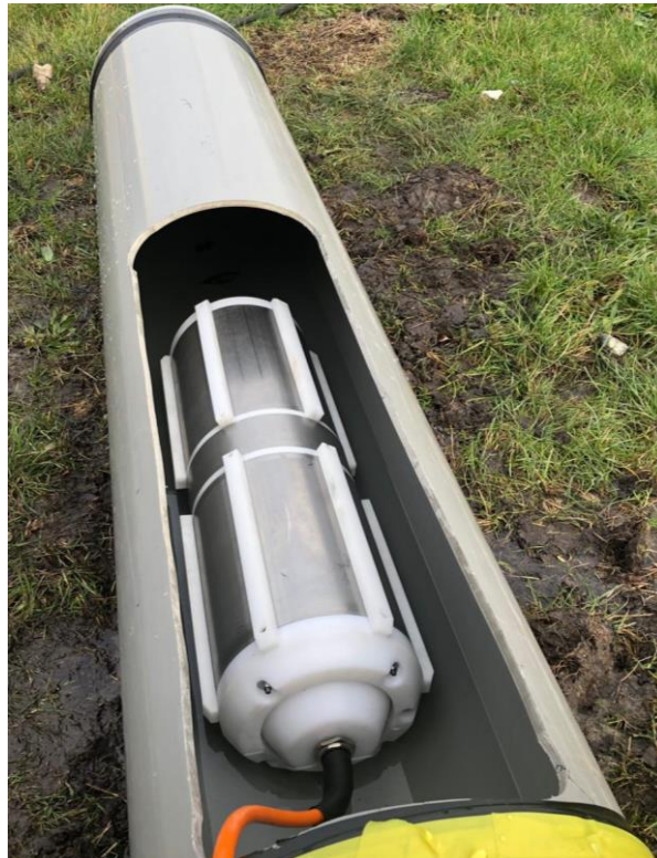
Figure 3: The FELL prototype 2.0 probe with casing in a PVC pipe 400 mm diameter
