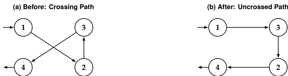
Figure 3.4: Illustration of the 2-Opt (intra-route) operator. (a) The initial route follows the sequence 1 \rightarrow 2 \rightarrow 3 \rightarrow 4 , resulting in crossing edges. (b) The operator reconnects the nodes to form the non-crossing sequence 1 \rightarrow 3 \rightarrow 2 \rightarrow 4 . Note that the segment between nodes 2 and 3 has reversed direction.
